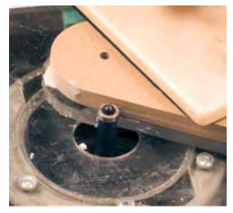
Using the same bearing-guided flush-cutting bit, the outside of the jig is trimmed neatly to the template.
