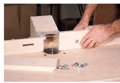
Attach the fence faces using  $3^{\circ}$ " roundhead machine screws, a star washer, flat washer and wing nut. I tried using hex-head bolts but switched to screws because a screwdriver can be used and makes a more secure attachment with less trouble.
