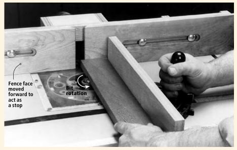
You also can use a fence as a stop to prevent creep. However, the fence must be precisely parallel to the miter-gauge slot and you must be feeding the workpiece with the rotation of the bit to pull the piece against the fence.
