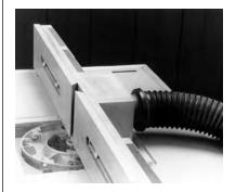
If possible, make sure your router table has a dust collector to minimize airborne dust as you work. On the table seen here, the collector is part of the fence.
