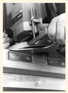
Most base-mounted guides will follow either straight or contoured edges, depending on the shape of the guide. Here, a straight guide – which looks like a small fence – rides along the edge of a board.
