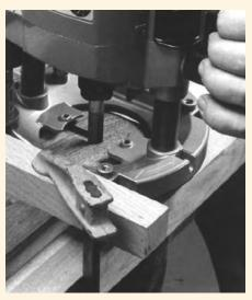
The depth stop will halt the bit at the proper depth. Secure the height clamp and rout the mortise, keeping the router against the guide.
