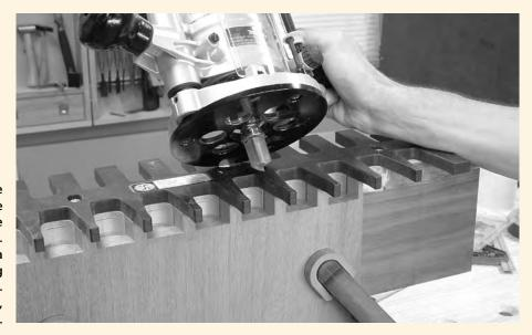
When using a fixed through-dovetail template you can't change the size and position of the tails and pins. Rout the tails first, using the tail template, a guide collar and a dovetail bit. Then you can switch to the pin template and a straight bit. Fit the pins to the tails by moving the template forward or back on its holder. This will change the size, but not the location, of the pins.
