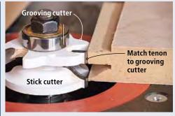
2 Tighten the top of the tenon. The next step is to tighten up the joint between the tenon and the cope. Using your test cope piece as a guide, mount the grooving cutter and shim it as best as you can to match the tenon on the test cope piece.
