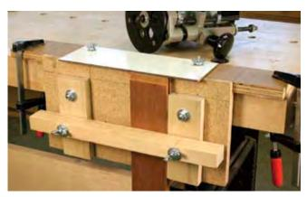
This clamping jig lets me quickly make the tenons without adjusting the router setup. The work is clamped vertically below the Masonite guide piece.
