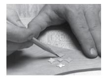
To inlay a shape, first trace the outline on the wood surface. This can be a difficult task, particularly if the design includes several small shapes. To keep wooden shapes from shifting as you trace around them, stick them to the surface with double-stick tape. To keep hard, dense materials in place, glue them to the wood surface with white (polyvinyl resin) glue. The adhesive won't hold the inlays in place permanently, but it will secure them long enough to trace the outline.
