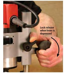
Location and direction of the plungerelease lever is also important. Some, such as the Milwaukee shown here, release when pushed down. Others lock when the lever is pushed down.
