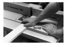
When routing the end of a narrow workpiece on a router table, use a large square scrap to guide it along the fence. The scrap not only holds the work perpendicular to the fence, it also backs up the wood so it won't tear out at the end of the cut.
