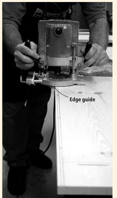
Rabbets and grooves are pretty easy to make with a hand-held router. Here you see a router cutting a  $\frac{1}{4}$ "-deep groove with a  $\frac{1}{4}$ " straight bit and an edge guide.
