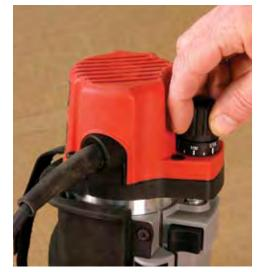
The Milwaukee's fine adjustment on its fixed base was the favorite of the routers tested.
