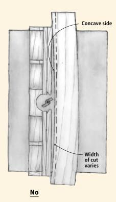
If you turn the concave side toward the fence, the cut will be narrower toward the middle of the board than it will be at the ends.
