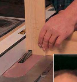
(Above) A dado stack in your table saw is all you need to make the template for routing the pins. Don't worry too much about tear-out on the backside of the work. It's just a template.
