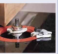
Get familiar with the parts. Many twobit sets work great right out of the box; others make joints that are too loose or too tight. You can fix the problem, but you're going to have to disassemble the bits to adjust the cutters. Plan on this taking an hour or two of your time. It's a pain, but remember you won't have to do this again until you get your bits resharpened.
