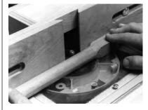
By rounding over the four arrises of a square workpiece (where the edges and faces meet), you can make your own dowels on a router table. The width and thickness of the workpiece should be precisely twice the radius of the bit. As you rout the four edges, leave about 2" of stock uncut on either end of the piece to keep the work stable on the router table.
