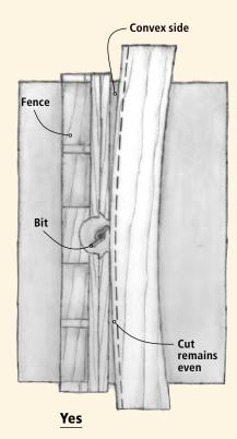
If your workpiece is warped or bowed – even slightly – keep the convex side of the bow against the fence or straightedge as you cut. The width of the cut will remain the same from one end of the board to the other.
