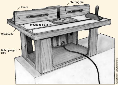
If you don't have room for a standalone table, you can customize other fixtures already in your shop to hold a router. A workbench, a table saw or a radial-arm saw all can pull double-duty as a router table.
