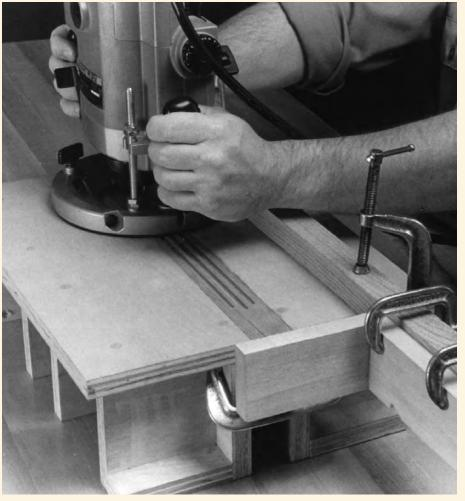
A flute is just a half-round groove – the opposite of a half-round bead. Often, it's blind at one or both ends. Use a veining bit to cut the flute and a straightedge to guide your router. If the flute is blind, it helps to have a plunge router. Attach stops to the straightedge to halt the cut when the flute is the correct length.
