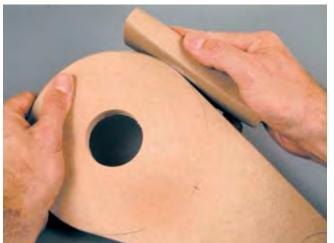
With everything cut, bored and sized appropriately, the last step is to clean up the edge so that it's smooth. A block and sandpaper can do most of the work, but an edge sander (if available) will be much quicker.
