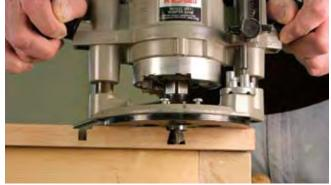
As you slide the router along the edge, the guide bushing and dovetail bit will enter the dado together.
