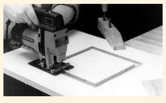
Next, make the router opening by cutting the inside edges of the groove with a jigsaw. This groove will then form the ledge to hold the plate.
