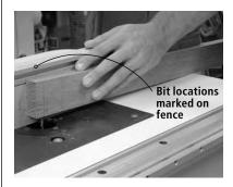
Stopped grooves or dados can be made safely on the router table by first marking the bit location (both sides of the bit profile) on the fence, then carefully lowering and raising the piece for the cut using the end of the board opposite the cut as a fulcrum.
