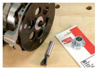
The 3/4" outside-diameter guide bushing must be reduced in length to protrude less than <sup>1</sup>/8". This modification allows the base of the router to lay flat on the workpiece.
