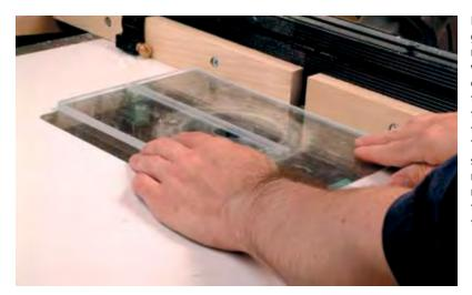
Running the grooves for the mounting hardware in both the offset base and the extension is a two-step router table operation. The  $\frac{1}{4}$ " - deep stopped groove is run first, using the router table fence to locate the slot in the center.
