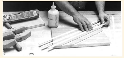
Next, test-fit the banding in its recess. When you're satisfied with the fit, spread glue in the recess and press the banding in place. Wipe away any excess glue, place a piece of wax paper or plastic wrap over the banding and clamp a straight, thick board to the piece over the covering. The board helps distribute clamping pressure evenly, and the covering keeps it from sticking.
