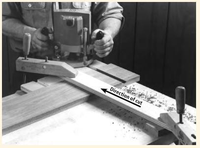
Lay out the joints on the workpiece. Place the jig across the wood, butt the crossbar against an edge or end, and line up one of the dados with the layout lines. Then clamp the jig to the workpiece and cut the joint using the straightedge to guide the router, just as you did when you made the dados in the crossbar.
