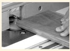
When you're ready to shape your workpiece, first cut the end grain along the ends ...
