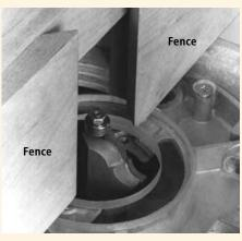
When properly used, a fence guides the work and also protects you from the bit. Even when using a bit with a bearing guide, align the fence faces even with the front edge of the bearing and adjust the fence gap as tightly against the bit as possible. • Let the fence surround the unused portion of the bit.
