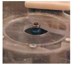
I used a bearing-guided roundover bit to soften the bottom edges of the jigs to protect the wood from scratches and to protect the slightly fragile edges on the jig itself. For the rest of the edges, sandpaper works fine.
