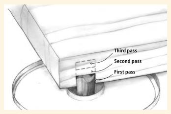
• Take note of the wood grain direction and rout with the grain as much as possible. When you must rout across the grain, back up the wood where the bit will exit. This prevents the bit from tearing and chipping the wood.
