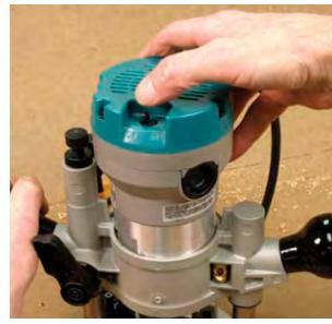
For some switches, such as on this Makita, it's necessary to remove one hand from the router to turn it on or off.
