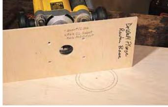
A larger base for the router was the ticket for bridging the open areas left by routing out the plywood for the router's base. It was also used as a small circle-cutting jig for the tabletop and plastic inserts. Use the same cutter and it's easy to keep track of dimensions for cutting inside or outside circles.
