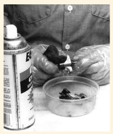
To remove the pitch from a router bit, soak it in lacquer thinner or spray it with oven cleaner. Give the solvent a moment or two to work, then wipe off the bit with fine steel wool.
