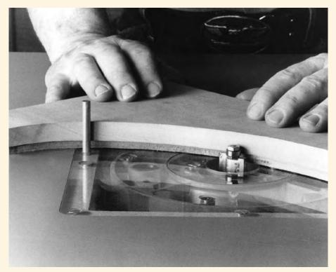
When cutting a joint in a contoured edge, use a guided-bearing bit to follow the contour. A bearingguided rabbeting bit will neatly cut a rabbet in an irregular edge, while a spline cutter will likewise make a groove in an irregular edge a simple task.
