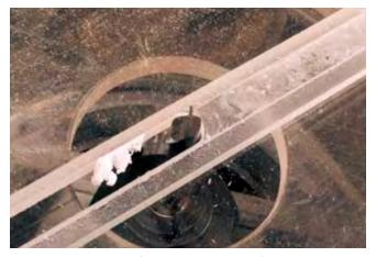
The through-groove is cut afterward, again using the fence as a guide. You may be able to switch bits in the router without moving the fence and keep everything perfectly centered. If not, double-check the through-groove's location.
