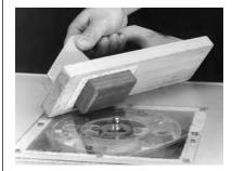
When cutting small pieces on a router table, be careful to keep your hands and fingers clear of the bit. You may wish to secure the stock to a push block or a large scrap with double-stick tape (as shown above) to rout it safely.
