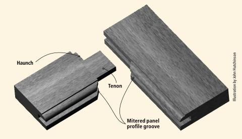
This door shows a complex version of a rail-and-stile joint. The haunch fills the groove left by the bit. Also, the decorative moulding is mitered at the corner for a classy finish.
