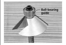
You may still find a few piloted router bits out there, but ball-bearing router bits are far superior, and have all but replaced the older design. Upkeep is easier on the ballbearing design because all you have to do is add a little lubrication from time to time.
