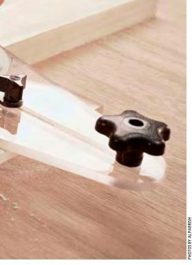
By swapping a few pieces of hardware, you can use this system as either a small (above, top) or large (above) circle-cutting jig, or simply as an edge guide. the offset base. With the extension added, you can expand the circle-cutting capacity up to a full 56" diameter.
