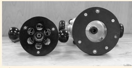
The 1<sup>1</sup>/<sub>2</sub>-hp router (left) has a base opening that is sized for bits appropriate to that size motor. The larger plunge router (right) has a 3-hp motor, appropriately sized for larger bits for panel raising or large profiles. This base has a larger opening to accommodate those bits.
