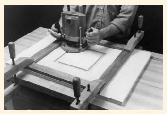
To cut the work surface for the mounting plate, first rout a square groove. Clamp a frame to the table to guide the router and cut the groove as deep as you want the thickness of the mounting plate.
