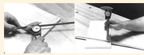
When inlay materials are thick, you can rout a recess to make the inlay "proud," then sand it flush. When inlay materials are thin, you risk sanding through them if you mount them proud. Instead, use calipers to measure the inlay thickness, then adjust the depth of cut to match.
