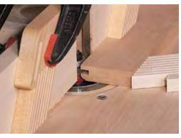
Using featherboards to keep your stock in place, press the stock into the fence and down onto the router table. Which profile you cut first isn't critical. Use test cuts to get your bits in the ballpark. I cut the stick first. For door construction, you can cut your stock to finish length, but I prefer to leave the stiles a little long for trimming later.
