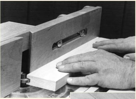
A tongue-and-groove joint requires two matching bits. Rout a groove in one edge of each of the workpieces, then change bits and rout a tongue in the other edge. You must carefully adjust the depth of cut for the second cut to match the first so the faces of the adjoining boards will be flush.
