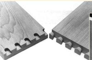
On half-blind dovetails (above), the joint is hidden from view on one side. This makes it ideal for the fronts of drawers and other applications where you don't want to see the joinery. Through dovetails (right) are visible from both sides and are often used for decoration, as well as joining.
