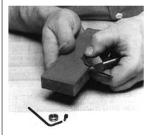
If your cutting edges seem dull, touch up the carbide flutes on a diamond stone. Sharpen only the inside (flat) surfaces of the flutes, leaving the outside (curved) edges alone. If you try to sharpen those, you might change the diameter of the bit.
