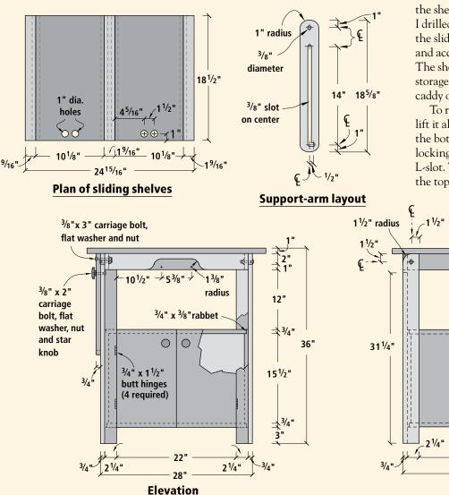
I routed a long slot perpendicular to the short one, then cleaned up the edges of the short slot with a file. When mounting the support arm to the stand, the short portion of the slot faces front.
