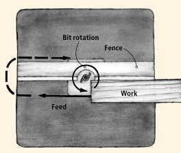
When a router is vertical under a table, the bit spins counterclockwise when viewed from above. Whether cutting the edge or interior of a workpiece, feed clockwise around the fence.
