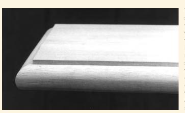
This tabletop will see a lot of use, so the woodworker who made it cut a thumbnail moulding in the edge. This relatively simple shape preserves the strength of the edge, while a more complex shape would weaken it and the edge would soon show the wear.
