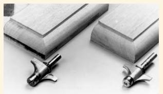
For best results, use guide bearings, rather than pilots or pins, which turn at the same speed as the bit and rub the edge of the workpiece. The friction causes them to heat up and burn the wood. Bearings turn independently of the bit and won't rub or burn the wood.
