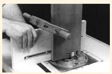
To use the jig, screw or bolt the mount to a miter gauge. Loosen the wing nuts that secure the face to the mount and slide the face sideways until the stop is the proper distance away from the bit. When the stop is positioned properly, tighten the wing nuts.
