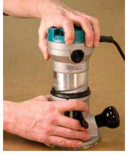
Routers without a fine-thread adjustment on the fixed base have coarse threads on the motor housing. Depth of cut is set by twisting the base in the motor housing.
