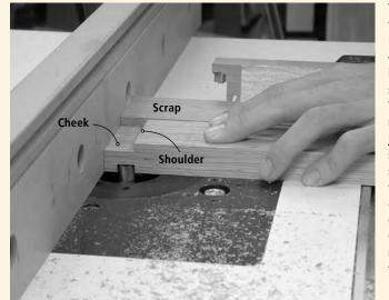
To make a tenon, cut two or more rabbets in the end of the board - these rabbets will become the cheeks and shoulders of the tenon. To fit the tenon to the mortise, cut the tenon just a bit large, then slowly raise the bit, shaving away a paperthin layer of stock on each cheek until you get the fit you're after. Guide the cuts with the miter gauge, using the fence as a stop.
