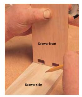
Now lay out the tails by tracing around the inside of your pins. A sharp pencil is key.
