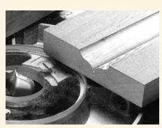
Point-cut bits with a complex shape, such as this pilotless ogee bit, cut a broad groove with an interesting shape. The sides of the grooves are mirror images of each other.
