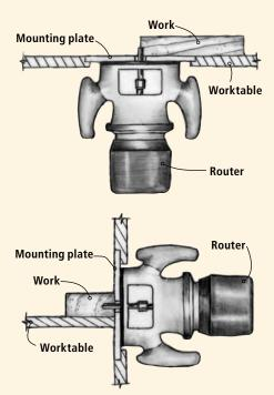
There are two common ways to mount a portable router and hold it stationary. You can mount it vertically under the work (top) or horizontally beside the work (bottom).
