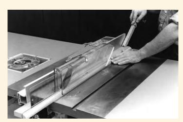
To make an applied moulding or picture-frame stock, cut the shape you want in the edge of a wide board, then rip it to the proper thickness, which I'm doing here on my table saw. Don't try to rout a shape in narrow stock – it may chip, splinter or kick back at you.
