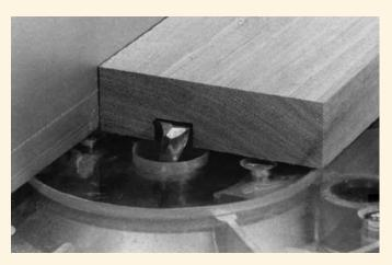
When routing dados and grooves, the joint ordinarily will be the same width as the bit. If you need to make a joint of a larger size, first make a cut that's somewhat narrower than the joint needed (left), then move the fence or straightedge to make a second cut (below), enlarging the joint to the desired width.
