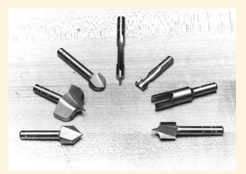
Most unpiloted router bits have either top-cut or point-cut flutes – flat or pointed cutting edges on the ends of the flutes as well as the sides. This feature lets you cut downward into the stock to make grooves, mortises and other cuts in the interior of a workpiece. For example, a point-cut beading bit (far right) lets you cut quarter-round and half-round shapes in the surface of a piece, not just on the arrises and corners.
