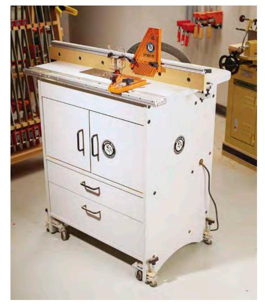
crown mouldings for furniture and architectural woodwork. In comparison, router bits are vertically challenged by the relatively short length of router-bit shanks. Even so, the largest routers don't have the heavy-duty bearings and horsepower to support and drive large bits through heavy cuts like a shaper.
