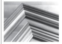
Instead of making multiple passes to create a complex moulding, just glue up several simpler shapes. The easiest way to do this is to "laminate" the shapes – or build them up in layers. But you can also "join" the shapes by cutting dados, rabbets or grooves in the moulding stock, then glue smaller strips of wood in these joints. The strips that you glue together don't have to be the same species – you can use contrasting wood, if you want.
