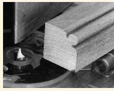
Make multiple passes with a beading bit to create decorative reeds and beads in the surface of a board. Because the beading bit is actually a small point-cut quarter-round bit, each pass cuts a 90° arc – one-quarter of a circle. Halfround beads require two passes. The corner bead or reed on this table leg requires three passes because it is three-quarters round.
