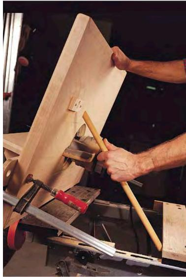
Once the tabletop is hinged to the Workmate's front board, it's easy to locate the the positions for the prop stick and stick bracket. Note the shop-made replacement board for the Workmate top.
