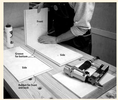
This drawer box is made pretty easily with rabbets. The front and back rest in  $\frac{1}{2}$ "-wide x  $\frac{1}{4}$ "-deep rabbets in the side pieces. The bottom slides into a  $\frac{1}{4}$ "-wide x  $\frac{1}{4}$ "-deep groove in the sides and front. The back is  $\frac{1}{2}$ " shorter than the front to allow the bottom to slide in.
