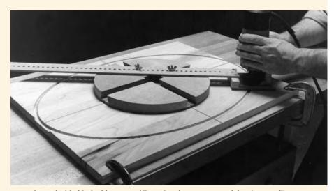
To cut the oval with this double-trammel jig, swing the router around the pivots, pulling gently outward. This slight tension will take any play out of the mechanical system as the pivots slide back and forth in their grooves. Make the cut in several passes.
