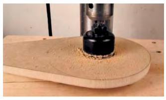
For the interior holes in the template, hole cutting saws, Forstner bits or spade bits will do the job. Make sure you back up the template to avoid blowout on the backside of the workpiece.
