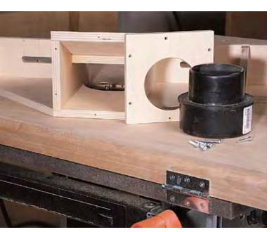
Inside view of the dust chute from the rear including the plastic 4" to 3" dust-collection hose adapter. Rout the 3" hole for the adapter with the circle-cutting jig or use a "fly cutter" in your drill press.
