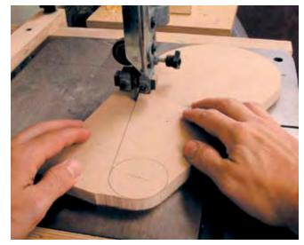
After transferring the template pattern to the template material, it takes only a minute to rough-out the shape on the band saw. Cut as close to the line as you can to keep clean-up to a minimum.
