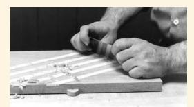
When the glue is dry, remove the board and the covering, then scrape away any glue that remains on the surface. But be careful – you don't want to scrape through the banding.
