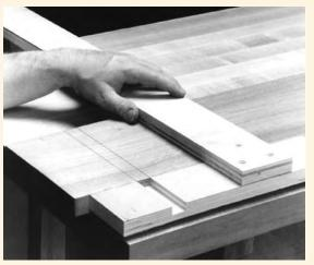
Before you can use this jig, you must cut dados in the crossbar – one on either side of the straightedge. Place the jig over a large wooden scrap and butt the crossbar against an edge. Clamp the jig to the scrap and cut the dados with a straight bit, keeping the router pressed against the straightedge. NOTE: Once you have cut these dados, you can only use the jig with that particular router and that bit. The dados won't line up with different tools.
