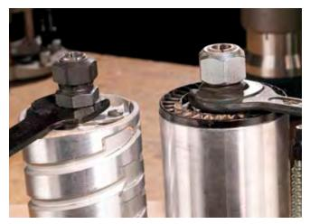
The large cast wrench of the Milwaukee (right) made for easy bit tightening. The thin stamped wrench of the Makita (left) tended to slip off the nut.
