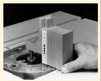
To use the gauge, set it to the desired height. Place it on the router sole or mounting plate with the arm over the bit. Raise or lower the bit until it touches the arm.
