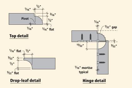
A great application for the rule joint is to install drop-leaf table hinges. You just need to make sure you think before you act. What seems normal – just placing the hinge barrel where the leaf and top meet, like a door to a stile – is totally wrong. As with all hinges, the location of the pivot point is the ultimate concern. With the drop-leaf hinge, the pivot point (the center of the pin) must be centered on the radius of the matching profiles.
