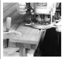
Whenever you're routing something, make sure that either your workpiece or your router is stable and secure – they can't both move. If you choose to move the router across the work, clamp the work to your bench. If a clamp interferes with the operation, rout up to it and turn the router off. Then move the clamp to an area on the workpiece that you've already cut and resume routing.
