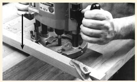
To rout a mortise with a plunge router, clamp a straightedge or guide to the workpiece and adjust the depth stop. (You also may use a base-mounted guide attached to the router.) Position the router over the work, holding the base against the straightedge (or the guide against the work). Release the height clamp and push the bit into the wood.
