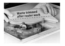
If a workpiece is very small, your hands may come too close to the router bit as you rout it. In this case, you have two choices – you can rout the work with a portable router using a commercially available foam rubber "routing pad" or double-stick tape to hold the work, or you can rout a portion of a larger workpiece and cut a small piece from it, as seen above.
