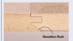
**RESULT:** Flush shoulders. At this point the joint made by these cutters would be pretty sloppy, as shown in the photo above. You can see, however, that the cut is flush on the shoulder (bottom) of the joint, which is the point of this important first step.
