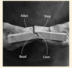
When both rule joint profiles are correct, the pieces should nest together with the top surfaces flush and a very small gap between the profiles.
