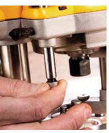
A fine-threaded nut at the end of the plunge rod makes fine-tuning depth settings simple and precise.
