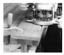
Whenever you're routing something, make sure that either your workpiece or your router is stable and secure – they can't both move. If you choose to move the router across the work, clamp the work to your bench. If a clamp interferes with the operation, rout up to it and turn the router off. Then move the clamp to an area on the workpiece that you've already cut and resume routing.
