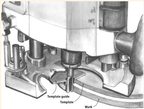
Template guides are designed to follow templates. As the guide traces the shape of the template, the bit cuts a similar shape in the workpiece. The routed shape is a little larger than the template, depending on the relative diameters of the bit and the template guide.
