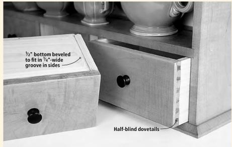
The drawer bottom in the drawer shown at left is  $\frac{1}{2}$ " thick but is beveled to slip into a  $\frac{1}{4}$ " groove, a traditional drawer construction method. Also, you can see the half-blind dovetails connecting the side with the front in the drawer at right.
