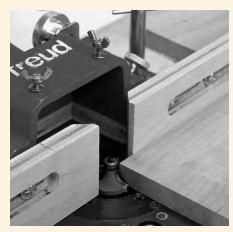
You can rout a rule joint using a simple cove bit. The bit height should leave a flat to match the mating profile's bead.
