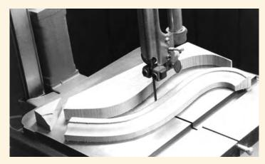
This safety consideration also applies to making curved mouldings, such as a classic "gooseneck" moulding. Cut the inside curve in the wide moulding stock, sand it so the curves are fair, then rout the shape in the edge.
