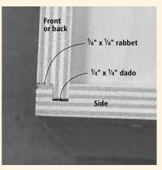
A simple and very common drawer joint in commercial furniture is the tongue-andrabbet (or dado-and-rabbet) joint. It's made by simply running a dado in the drawer sides and then rabbets on the drawer fronts and backs. Both operations are best made with a router in a table.
