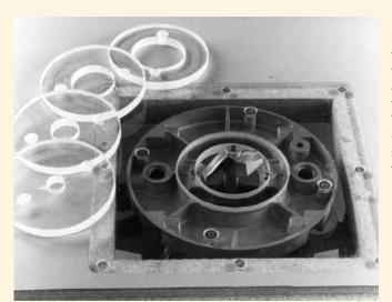
Because router bits can range in size from <sup>1</sup>/16" to 3<sup>1</sup>⁄4", you should drill the plate's opening about <sup>1</sup>⁄4" larger than the largest bit you own. Then you can make several inserts out of the same acrylic you used for the plate.
