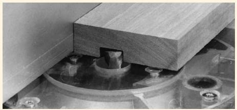
Because most basic joints are cut parallel or perpendicular to straight edges, you must guide the router or the work in a straight line. The best way to do this is to use an edge guide, straightedge, fence or miter gauge. You also can use a shopmade jig, such as the T-square Router Guide (which is featured on page 34 in Chapter One of this series).
