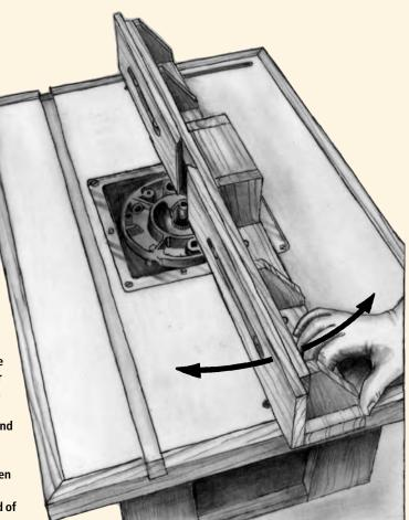
on the market are designed for use with fixed-base routers, which is fine, but you should choose a router with variablespeed control to take maximum advantage of the larger motor and available larger-diameter bits.
