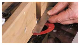
Setting up and using a cope-and-stick set of bits is relatively easy after the shimming is done. First, make sure the bearing on the bit is flush with the fence on the router table. Flushing the bearings makes sure that the profiles will match up. Use a straightedge that spans the two fences and tap the fence flush to the bearing. If possible, close the fence faces so there's approximately  $\frac{1}{8}$ " clearance on both sides of the cutter.
