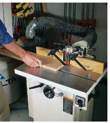
One of the advantages of the shaper is that its motor can run in reverse. This allows you to adapt to wood where the grain runs in a different direction. It also helps with wide, thick or odd-shaped stock.
