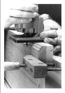
If you're routing the thin edge of a workpiece (such as when mortising), or if the workpiece is too narrow to balance the router easily, clamp a thick scrap to the work to provide more support.
