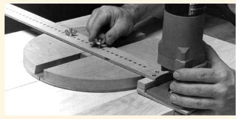
Swing the beam 90°, aligning it with the minor axis, and position the router so the bit is at the end of that axis. Center the major pivot over point Y and fasten the beam to it. The beam should now be fastened to both pivots. To check the setup, swing the router once around the pivots with the power off. The bit should pass over the ends of the major and minor axes.
