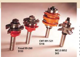
The three types of cope-and-stick bits. On the left is a matched set of cutters. One bit for the stick; another for the cope. In the center is a non-adjustable combination bit. You change from cope to stick by changing the height of the router. On the right is a reversible bit. After cutting the stick profile, you disassemble the bit and rearrange the pieces to cut the cope.
