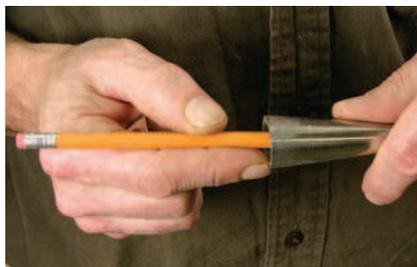
**Close is close enough.** Don't be fussy with an exact measurement for the depth of the socket; use your finger or a pencil as a gauge.
