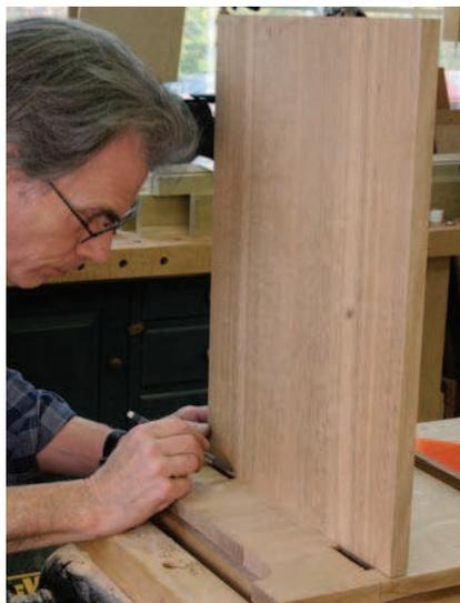
**Make your mark.** Wait until the mortises are completed to lay out the tenons on the cabinet top and bottom. Mark the locations from existing edges.
