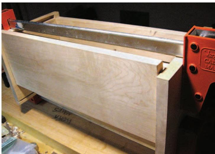
**Dado work ahead.** You can see the lid stops at this point; I will disassemble the tool chest and lengthen the 'L' shaped dado so, when open, the lid will be flush with the top of the sides.
