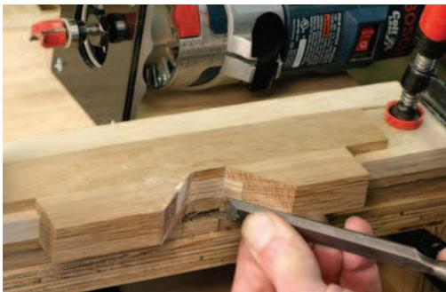
**Double duty.** This jig guides the bearing on a flush-trim router bit, then is used to guide a chisel to pare into the mitered corners.
