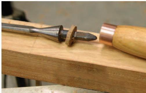
**Beneath the plastic.** Most plastic-handled chisels look like this inside. The ferrule keeps the handle from splitting, and a leather ring absorbs shock and fills the gap.
