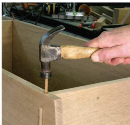
**Overkill.** The dowel reinforces the through mortise and tenon joint. It isn't needed, but it's a nice detail to include.
