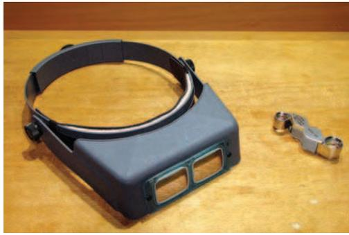
**Visual aids.** On the left is a Donegan Optivisor LX with a 10" focal length, which allows you to focus at least that close to your work. On the right is a hand-held multi-element magnifier, which is useful for getting a close look at very small items – such as when you're checking for grit scratches on blades while sharpening.
