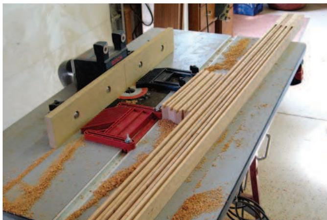
**A furrow for your panel.** A powerfully quick method to form grooves for the plywood panels is a sharp  $\frac{1}{4}$ " router bit and a nice router table setup.
