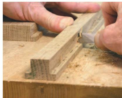
**Run in reverse.** The back of a chisel makes a great scraper, just the ticket for cleaning out the corner of rabbets.
