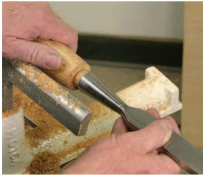
**Check it out.** A test-fit will tell you when the taper is correct.
