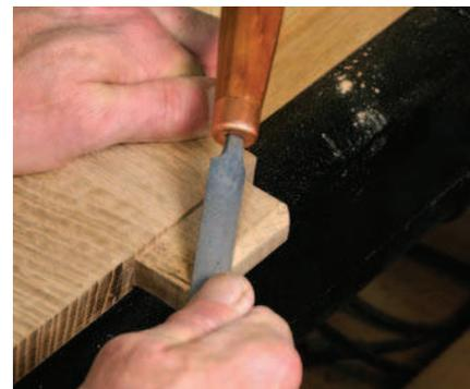
**Refined detail.** Make a slight bevel on the ends of the tenons before fitting. After a good dry-fit, mark the outside of the case on the tenon, then increase the bevels to end close to the line.
