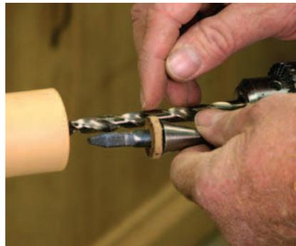
**A matter of judgment.** The depth of the hole should be somewhat deeper than the length of the tang. The end will be trimmed to fit.
