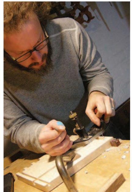
**Clean up.** A router plane completes the dado and cleans up the bottom.
