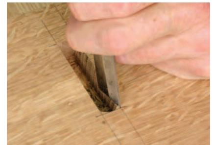
**And swing it.** Keep the back of the chisel pressed against the routed edge of the mortise and carefully rotate the edge into the corner.
