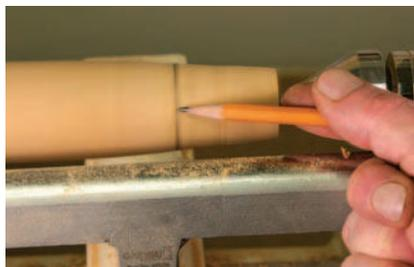
**Room to grow.** Leave some extra room to fit the taper. You will need to adjust the angle and the length as you fit the socket.
