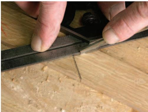
**X marks the spot.** The joints in the central mullion meet in the exact center. A knife cut along the lines will help to guide the saw.
