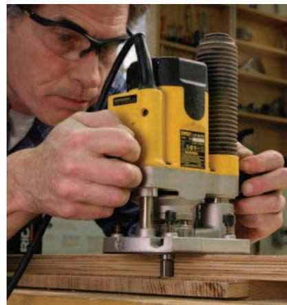
**Under control.** Cut the tenon shoulders first, using a straightedge and a bearing-guided router bit. Adjust the depth of cut in small increments to achieve the proper thickness.
