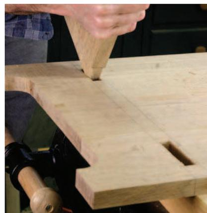
**First things first.** Test the thickness of the tenon by placing a corner of the shelf in the mortise. Aim for a tight fit at this point.
