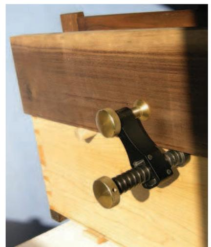
**Field jointing.** With the surface clamp in one of the front holes and a 3/4" dowel in the other, I can edge joint a board up to 24" long!
