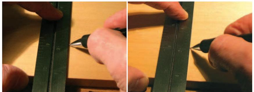
**Shadow play.** These photos show the value of moveable lighting. In the shot on the left, the marked line is invisible, hidden by the shadows of the square's blade and my hand. In the photo on the right, you can see the marked line.
