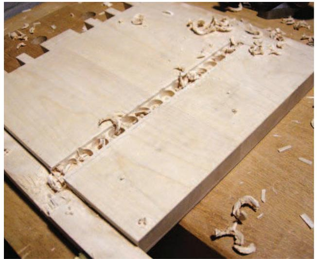
**A bit of choice.** You can use a bit and brace to remove the majority of the waste in a dado.
