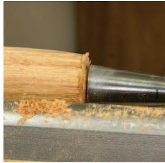
**Room for compression.** A small gap between the socket and the shoulder will keep the handle tight over time.
