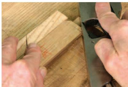
**Complex geometry.** Test the fit often while fitting the miters. Trimming one edge will lengthen or shorten an adjacent edge as well.
