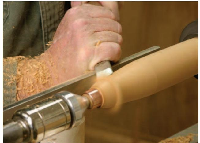
**Shaping up.** As the handle takes shape, carefully taper the end of the handle to the edge of the ferrule.
