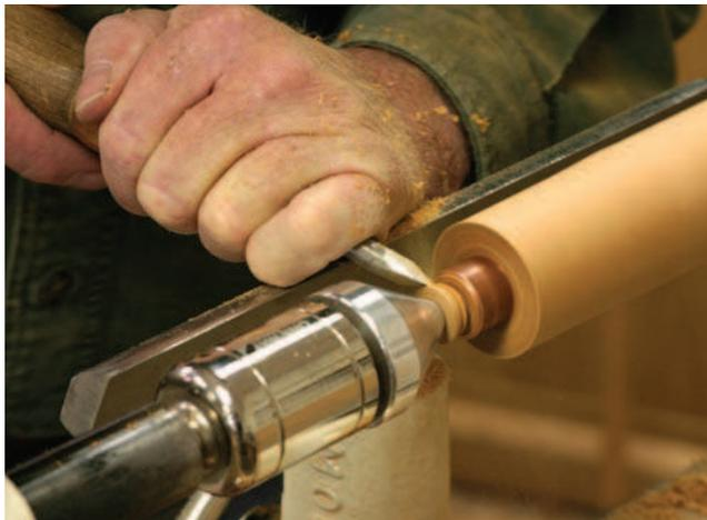
**Make it flush.** Remove the excess material beyond the ferrule, then move the cone center in.
