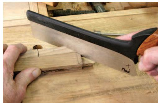
**Miters, too.** 45° cuts in the fence guide the saw to cut the short miters. Preserve the line at this point, and work down to it while fitting.
