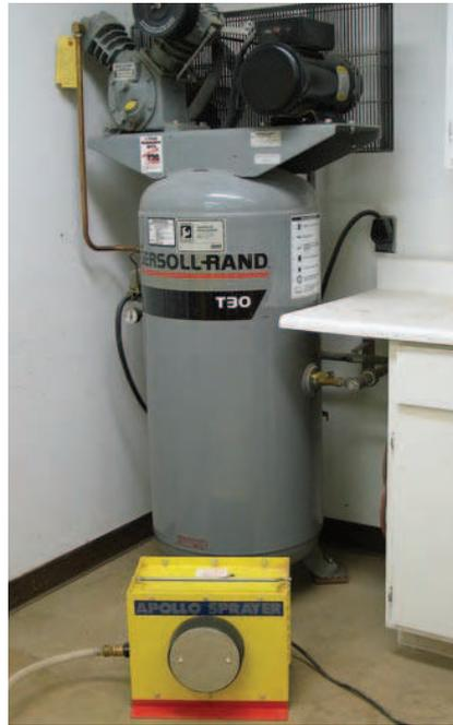
**Compressors.** Compressors big enough to supply spray guns sometimes come with wheels but are otherwise not easily portable. Turbines are small and fairly light so they are very portable. This compressor is 5 hp, produces 15 CFM and has a 60-gallon tank. The turbine is three stage – the smallest that atomizes adequately.
