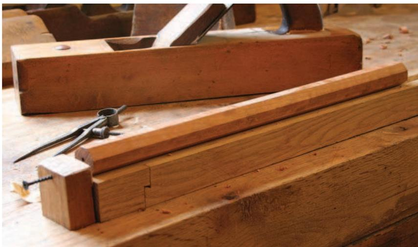
**Octagon.** Begin by making the bar stock. You can turn it round to  $\frac{3}{4}$ " on a lathe, or use a spokeshave to make an octagon, then true it with a  $\frac{3}{8}$ " hollow plane to  $\frac{3}{4}$ " diameter. Or, use a length of dowel.
