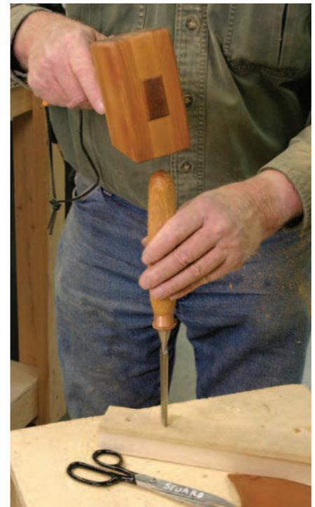
**A dab will do ya.** A small amount of epoxy in the hole will keep the tang connected. Place the leather over the tang and drive the handle on.
