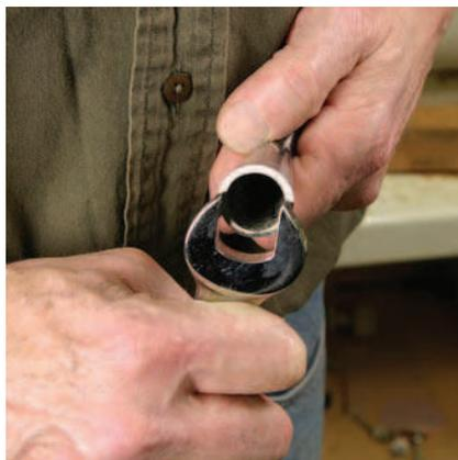
**An open-ended question.** Use a wrench to gauge the large diameter of the socket.
