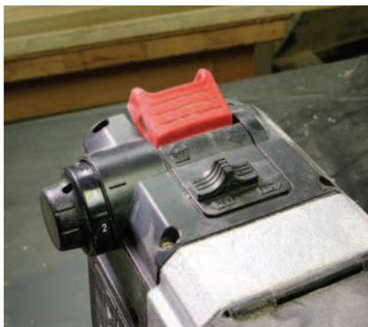
**Seals the deal.** If you're a lathe devotee, you know the value of being able to reverse the spin as you work. This Delta midi-lathe is the only benchtop lathe to offer this function.
