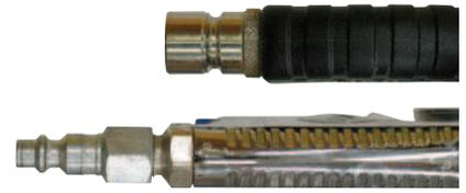
**Air inlets.** Quick-connect air inlets differ for compressor- and turbine-supplied spray guns. The air inlet on top is for turbine air; the one on the bottom is for compressed air.
