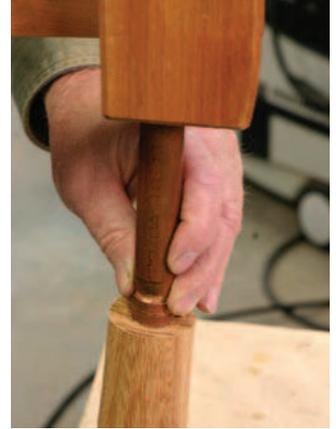
**Tap it in.** Use a length of pipe to drive the ferrule on to the end of the tenon. The ferrule will shave the last bit of the tenon for a snug fit.
