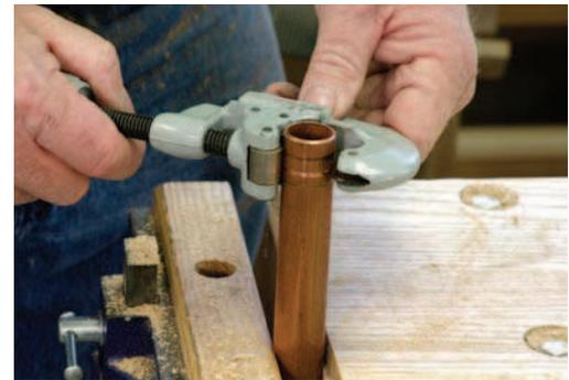
**The right tool.** An inexpensive pipe cutter makes a cut quickly and leaves smooth edges on the copper ferrule.
