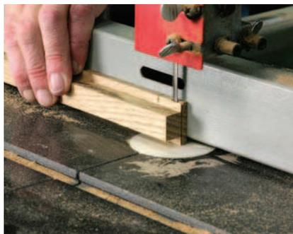
**Wasting away.** The band saw fence is set to leave just a sliver of material as the tenon cheeks are cut.
