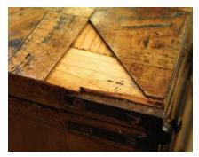
**4 The challenge.** Above the hinge you can see damage to the substrate that must be repaired so the veneer has something to bond to. Also, you can see that the veneer is considerably thicker than modern <sup>1</sup>/<sub>32</sub>"-thick veneer. Thick veneer is common on furniture made before the machine age. Veneer seems to get thicker the older the furniture.
