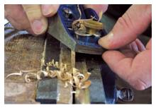
**No fastener is required.** The edges of the spring mechanism are planed to a dovetail shape to hold the spring in position as it's depressed. As pressure is applied to release the lock, the dovetailed sides push against the channel.
