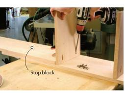
**Stop the creep.** Use a clamp and stop block, or in this case one of the bookcase sides, to keep your shelves from inching forward as screws are driven.
