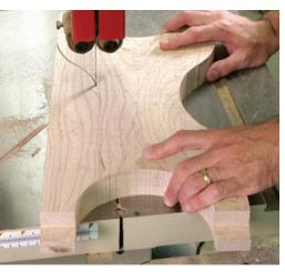
**Cutting curves.** These curves actually are more than eye appeal. They are convenient places to grab the board jack to slide it or to sneak a clamp into.
