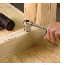
**Ratchet to attach it.** Use  $\frac{1}{2}$ " lag bolts to secure the base to the top. The pilot hole for the lag bolt should be the diameter of the bolt minus its screw threads.
