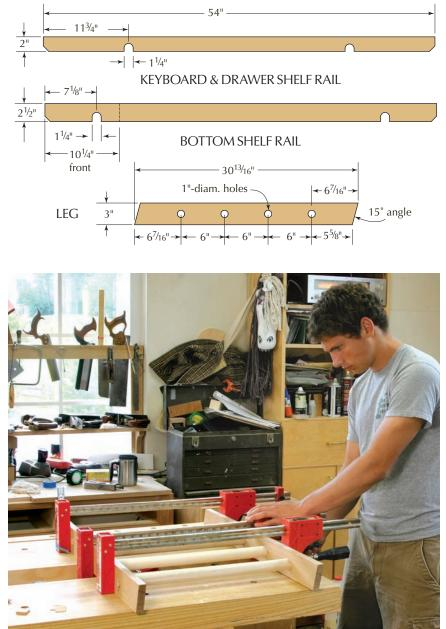
A reason to hide. I used liquid hide glue to allow more time to assemble the rungs and legs.
