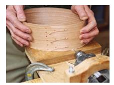
**11 Drill for pegs.** After the oval board is in place and sanded flush, drill the perimeter every 2" to 3" for wood pegs. This drill jig locks a spare drill to a board with a front table the right height to center the hole on the <sup>1</sup>/<sub>4</sub>" board inside.
