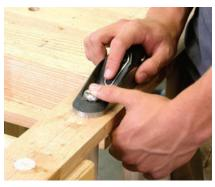
**New block for the kid.** A few passes with a block plane levels the ends of the tenons and wedges to the surface of the legs.
