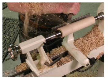
*Live center.* A live center with a ball bearing is one of the first accessories to get. It will reduce friction at the tail stock end.
