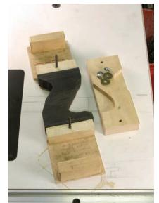
**3** Now rout. After you've cut to <sup>1</sup>/8" outside your marked shape, reinsert the blank and rout to final rough shape.
