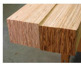
**Ripped and ready.** We began by ripping down the LVL 2x12s we needed for the benchtop and were surprised by how easily the material cut on the table saw with a combination blade.
