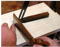
It's a compound cut. Use a bevel gauge, set to the angle planed on your key, to align your saw as you define the dovetailed channel. After the edges of the channel are sawn, use a chisel to waste out the material.
