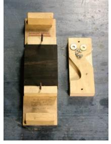
**2 Snug fit.** Make sure your tote blank fits snug between the holding blocks in the jig before tracing the tote's shape onto the blank.
