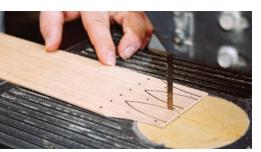
**1** Fingers. Profile the finger design to rough dimensions before final trimming with a utility knife. The locations for copper tacks are drilled at this time, too.
