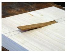
A different application. A spring lock is fit into a drawer bottom. From here, it's easy to fine-tune the fit so the lock catches the drawer blade and holds the drawer closed.
