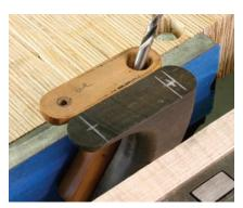
**6** Work from the original. Use the original tote to locate the proper angles and holes for attachment.
