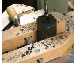
**9 Prep your knob blank.** Drill a hole that's a bit more narrow than needed – you'll enlarge the hole after turning the knob.
