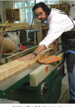
Jointing with carbide. Our jointer has a carbide-insert cutterhead, and it had no problems dealing with the glue in the LVL. I was more worried about the planer, which has highspeed steel knives.
