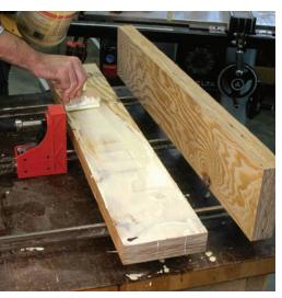
Joint and glue. Joint the inside face of each of your leg pieces and glue them together. When the glue dries, joint and plane the legs to their final thickness and width. Planing the legs to width ensures they will all be consistent.
