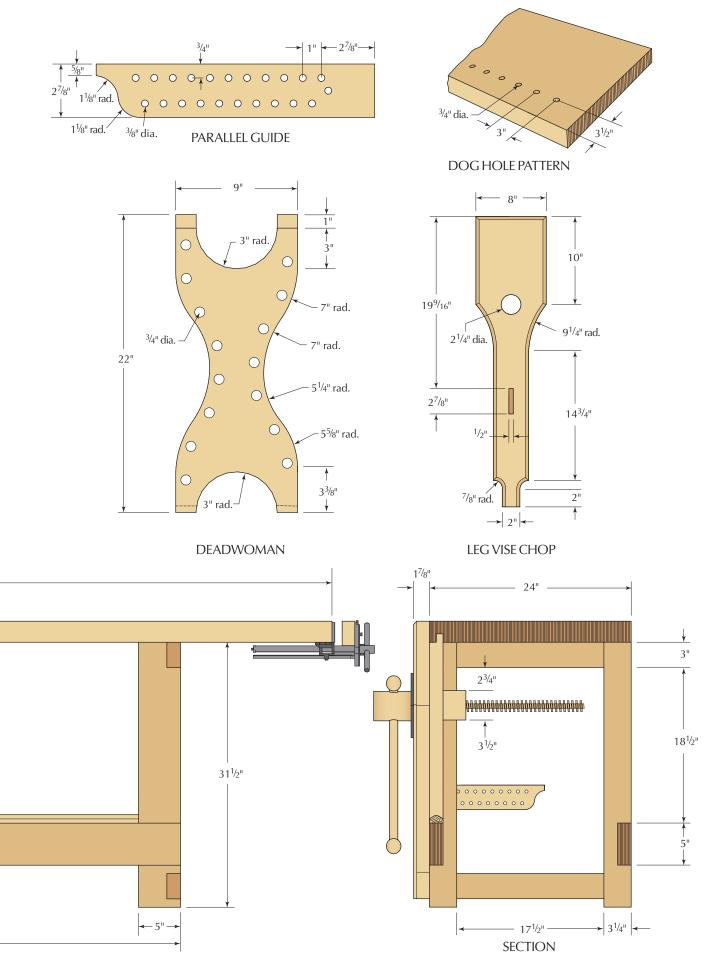
We used yellow glue through most of this project and didn't have any problems. When gluing LVL made using yellow pine, we recommend you keep it clamped at least five hours. Yellow pine has resin that resists glue penetration.
