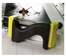
**5 Round over.** Place the tote blank in a small parts holder and use a roundover bit to shape the edges, then sand smooth.
