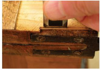
Straight edges. Again, it's always easiest to work with straight edges. So I'm cutting one using a chisel.
