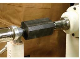
**10** *Turn.* Place the hole at the top of the blank over the drive center, and the smaller hole on the live center; turn the knob.
