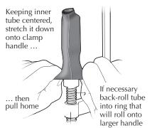
to remove it. In its ringed form, it will then easily roll onto a somewhat largerdiameter handle. For smaller-diameter handles, use a slightly narrower tube. You can often get old tubes for free from your local bike shop.
