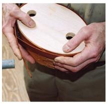
**Shapers.** Once tacked, wood corks called shapers are put in both sides to hold the box shape for one to two days of drying. The 10° edge bevel and the holes for ventilation are a hallmark of this piece of bench equipment that is key to the Shaker system of production. The top band is wrapped on the box itself. It will be tacked then returned to the box for drying. Note that the direction of the band finger matches that of the bottom band fingers.
