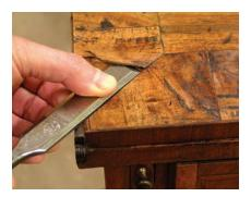
**2 Removing excess.** It's often possible to pop off the waste veneer as I'm doing here. When I meet resistance, I can usually overcome it if the glue is hide glue by using a syringe to insert a little denatured alcohol under the veneer. The alcohol crystallizes the glue, making it easier to separate.
