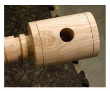
**Two garter grooves.** This wooden vise screw has two garter grooves. One is by the hub (for exterior garters) and the other is a little bit down the shaft (for interior garters).
