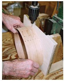
**12** Alternate approach. An alternative drilling method makes use of a drill press. The jig, which is shaped like a bookend, creates a vertical drilling station.
