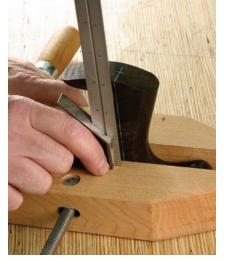
**T** Handscrew helper. A handscrew can securely hold the workpiece at the required angle for drilling.
