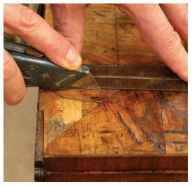
**1** Straight edges. It's far easier to shape a patch when you're dealing with straight rather than curved edges. So, if possible, I always try to straighten the edges before fitting my patch.
