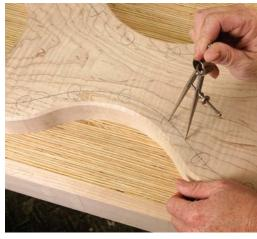
**Walk it off.** Dividers are the absolute best way to space the holes in the deadwoman. To offset the holes, simply bore a hole at every other mark left by the dividers.
