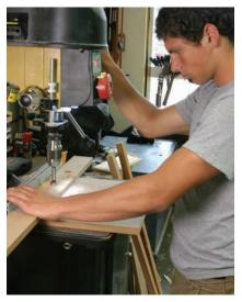
Holes in a row. Careful layout and setup of the holes in the legs makes for easy assembly and sturdy construction.
