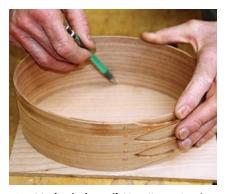
$\begin{array}{c} \textbf{B} \quad \textbf{Mechanical pencil.} \text{ Here I'm tracing the} \\ \text{oval on the } {}^{1}\!\!{}^{4}\text{" boards used for tops} \\ \text{and bottoms. A mechanical pencil will ensure} \\ \text{accuracy of this line.} \end{array}$
