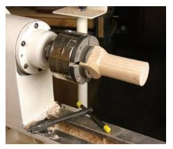
Versatile gripper. A four-jaw chuck will hold nearly anything, round or square, securely for turning. It also makes mounting work quick and easy.
