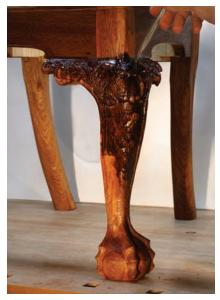
Wipe on, wipe off. I mixed burnt umber dry earth pigment with linseed oil and applied it with an acid brush. I wiped off the excess to highlight the high spots. The goal was to darken the knee and foot, where the exposed end grain was most pronounced. What I have here essentially is slow-curing oil-based paint.
