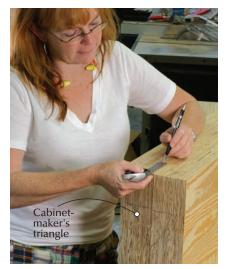
**Triangles and squares.** Note the "cabinetmaker's triangle" scrawled across the tops of the four legs. This helps you keep all the legs oriented as you mark out the half-lap joints for the stretchers.
