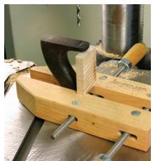
**8** Support. Place a support block underneath as you drill the attachment hole in the back of the handle – otherwise, it could break off.
