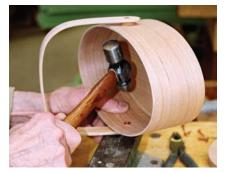
**Peen.** Peen the rivet until the handle is secured and will stay put.
