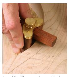
A special marking gauge. Because I do a lot of work with chairs, I have this marking gauge with a special fence that allows it to follow curves. If you don't have a gauge like this, it's easy to modify your standard gauge. Take some <sup>3</sup>/<sub>4</sub>" dowels, plane a flat on them and glue two short sections to the back of your fence. Turn your fence around and you'll have a gauge that does two operations.
