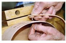
**14 Rivet sequence.** The rivet sequence is: copper trunk rivet, handle,  ${}^{3}/{}_{16}$ "-thick wood spacer, the box side in which has been drilled a  ${}^{5}/{}_{32}$ " hole, the copper washer for the inside end of the washer.
