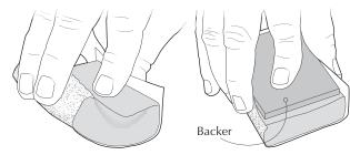
Bend sanding pad to desired contour
