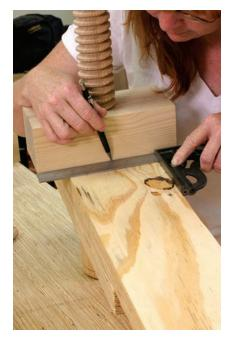
**Snug, square and traced.** Put the vise screw through the 2" hole and snug up the vise block on the backside of your leg. Square up the block then trace its outline on the leg.
