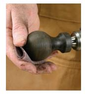
**12** Screwed on. Use a ground-down flathead screw through the knob to secure it to the lathe for final sanding.
