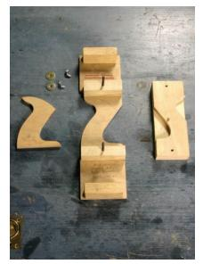
**1 Routing jig.** This jig, which holds the tote blank for routing, is made from scrap <sup>3</sup>/<sub>8</sub>" birch plywood, poplar and pine.
