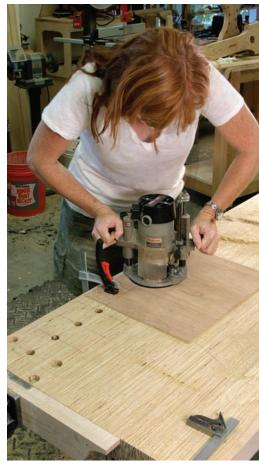
**More nasty dust.** The  ${}^{3/4}$ " upcut spiral bit and template makes short work of this operation. Lay out all your holes on the benchtop, then position the template and make your plunge. The template is marked with crosshairs that align things with your layout marks.
