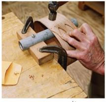
**Tacks.** Small copper tacks <sup>1</sup>/<sub>16</sub>" longer than the two thicknesses of veneer are used to clinch the lap. No glue is used. The wood cradle secures the pipe anvil to the bench.
