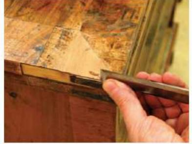
10 Trimming. With the top surface of the patch leveled, I trim the end using a chisel because of the difficulty of getting a handplane into the narrow area above the hinge. Notice the missing veneer to the left of the hinge. I popped it off (by inserting denatured alcohol) to make the shaping and trimming of the patch easier. With the patch trimmed flush I will reattach the veneer so it covers the edge as it originally did.
