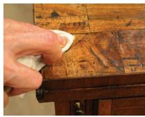
**3** Cleaning up. Though it's possible to reglue right over old hide glue using hot hide glue, it's best to clean off the old crumbly glue (and whatever contaminants, such as wax, that might be on the surface) before gluing the patch. Here I'm washing off the old glue with hot water. All contaminants come off with the glue.
