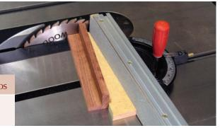
Use the miter gauge to square the short edge of an approximately 10" x 12" piece of  $^{3}/_{4}$ " MDF. Rotate the miter gauge clockwise and lock it at the desired dovetail angle. Holding the same edge as before against the miter fence, crosscut away a narrow wedge, about 2" wide, tapering to about  $^{1}/_{2}$ ". Glue sandpaper on the angled edge.
