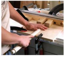
Take it for a spin. Tenons are formed on the ends of the rungs by rotating a dowel over the router bit.
