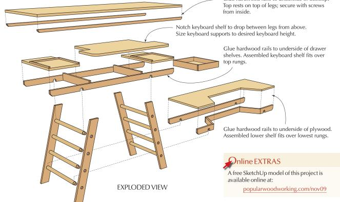
drilled the holes with a Forstner bit at the drill press, using the fence to center the holes in the legs.
