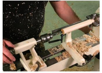
**Dead center holes.** The addition of a Jacob's chuck allows you to drill holes in the end of a spindle.
