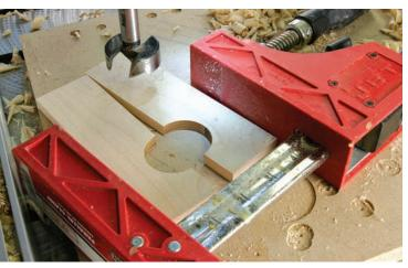
**Can't-miss garter hole.** Clamp the two halves of your garter together and bore the hole right through them. Our garter hole needed to be  $1^{5}/8^{"}$  in diameter to match the dimension of the shaft of the vise's screw.
