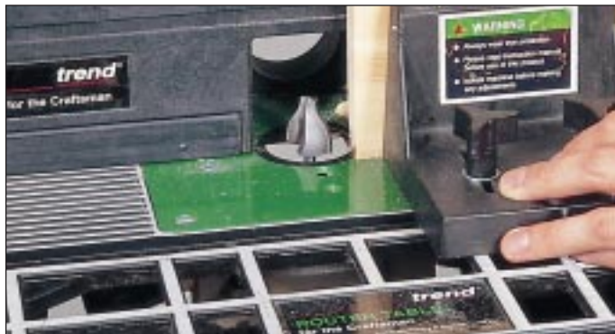
Positioning the vertical front support block
