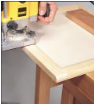
Edge moulding the glued panelled door using a ball bearing guided Ovolo cutter.
