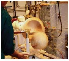
Photo 17. This photo was taken just as the second core was cut loose and popped out of the bowl
