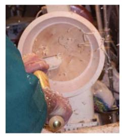
Photo 20. Here Hal is finish turning the inside of the salad bowl with fairly aggressive cuts.
