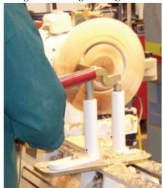
Photo 14. Here the coring tool is starting to cut the smallest core.
