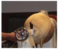
Photo 3. Here Hal has finalized the outside shape and if finishing the tenon (foot) that will be held in a chuck during the coring process. It is important that the foot on the bowl be at least three inches and preferable four or five inches on larger blanks. My experience with making only about two inch tenons is that they lead to disaster. Every 2" tenon I've used has resulted in a dismounted blank while coring.
