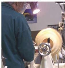
Photo 2. In this photo Hal is defining the shape of the outside of the potential bowl. It is very important to turn the outside to near final shape before starting to core because this helps in the selection of which of the cutters to use for the first core. This is especially true if you are using the McNaughton Center Saver System.
