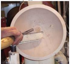
Photo 21. Carefully he makes the final cut to the center of the inside of the bowl. This is the cut in which you can tear out a chunk requiring additional passes to clean up the bottom, which can be very bad if you've already turned the wall thickness to the planned final thickness.
