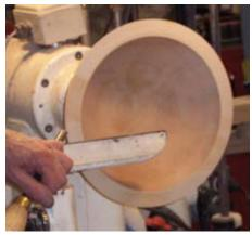
Photo 19. The bowl has been mounted in the chuck and the top of the rim is being final turned to remove all traces of the warping from drying.
