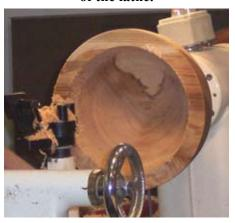
Photo 9. This photo was taken just after the core had been removed. Hal noted that he likes to clean up the inside of the bowl before removing it from the lathe and setting aside for drying.
