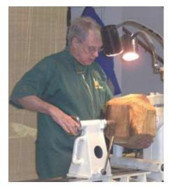
Photo 1. Hal Johnson began the demonstration by mounting a roughly shaped blank on Jack's Oneway 24-36 lathe and prepared to turn it round.
