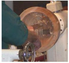
Photo 10. Here Hal is making a final pass on the inside of the cored bowl.
