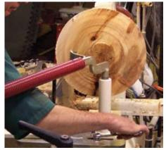
Photo 13. Hal started with a new blank that had been trued and had a foot turned for the chuck. In this photo, he is setting up the Oneway system. He is positioning it to remove the smallest core first.
