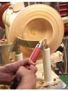
Photo 16. Starting the next core out. Using this system it is fairly easy to maintain the wall thickness of the cores that are being removed.
