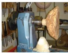
This balancing system is especially designed to be mounted on the outboard side of your lathe and is suited to do out-of-round off-centre work.
