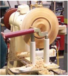
Photo 15. The coring on the smallest core is nearly done. Hal cut it until it started to wobble and then removed the core with his hand.
