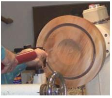
Photo 8. Here Hal is continuing to deepen the cut toward the center of the bowl blank. It is important to stop as the cut begins to approach the bottom to see if the core can be moved. It is often better to break off the tenon of the core rather than have it cut loose and be thrown somewhere. Although one can continue to cut until the core actually comes out on its own and it will generally fall on the far side of the lathe.
