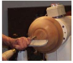
Photo 11. In this photo, the core from the previous bowl has been mounted on the lathe for truing up the outside and turning a new foot for this bowl.
