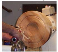
Photo 7. Hal said that his experience with the McNauthton system indicates that it is best to remove the largest core first, because the largest bowl is the most valuable. Working from the center out, it is possible to accidentally ruin the large bowl by cutting too deep on the other cores. Since this bowl blank is freshly cut wood he is leaving a wall thickness of at least 10 percent of the diameter, which will generally leave enough wood for final turning after the bowl has warped when drying.
