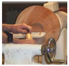
Photo 6. Although the center of the smallest bowl to be cored can be removed with the coring tools, Hal indicated that his experience was that is was easiest to simply turn away the center of the smallest bowl, unless the wood was a very expensive exotic wood that you would want to create a very small bowl to use all of the wood possible.
