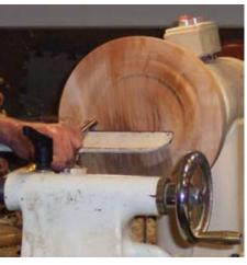
Photo 5. Truing the face of the bowl blank in preparation for coring. It is important for the face of the bowl to be smooth and flat for best coring operations.
