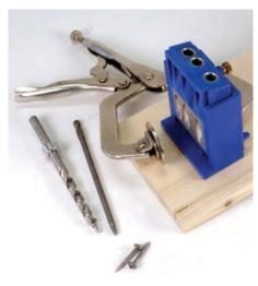
A pocket-hole jig allows you to join two pieces of wood without clamping. The only real downside is the fact that you have to conceal the holes made by the stepped drill bit.
