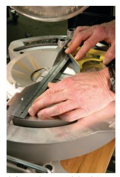
The fences on these saws can be bent during assembly. When you get your saw out of the box, check the fence with your square to ensure it's straight. If it's not, take the saw back and exchange it. A bent fence is almost impossible to fix and will cause a lifetime of headaches.
