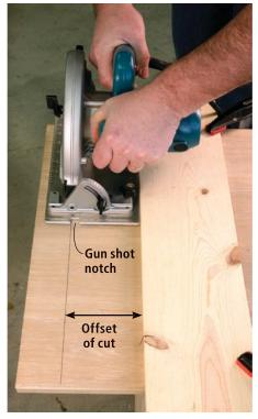
Clamping an auxiliary fence to the workpiece is an excellent way to achieve a straight cut, so long as the fence is also a straightedge. Notice the "qun shot" notch used for freehand cutting.
