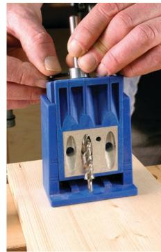
Setting the depth of the stop collar is simple. With one hand, you can push the collar down on the jig and hold the tip of the bit about <sup>1</sup>/<sub>8</sub>" above the jig. Use your other hand to tighten the set screw on the collar.
