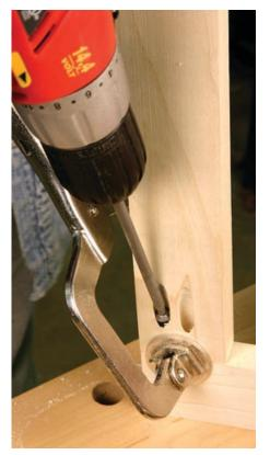
The long driver bit that comes in the kit keeps the drill chuck away from the wood.
