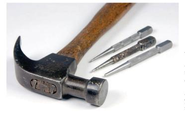
A good woodenhandled hammer and a few nail sets can serve you for a lifetime. Avoid the fiberglass and metal hammers. They are not as forgiving on your joints (as in your shoulder and elbow).
