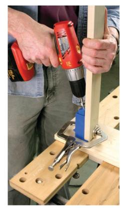
Use the high speed setting on your drill to make the pocket hole.
