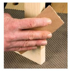
Always "break" the edges of your work before finishing. This makes your project nicer to the touch and makes your edges less susceptible to damage.
