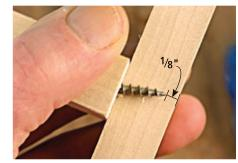
Hold a piece of scrap against the piece with the screw in it. Check to see that the end of the screw is about  $\frac{1}{8}$ " away from the surface.
