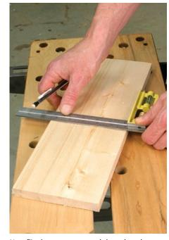
Now flip the square over and show the ruler to the line. If your square is true and your line consistent, then the line and the ruler should be perfectly parallel. If the line and the ruler don't match up, try the operation again before you reject the square — it's easy to trip yourself up when checking your square.
