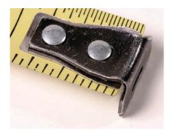
The hook should move in and out. The distance it moves should be equal to the thickness of the hook itself. Tweak the hook with pliers until the tape consistently measures inside and outside measurements.
