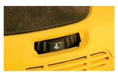
Generally, the variable-speed feature is unnecessary on a random-orbit sander. The only time I've slowed down the tool is when I was dealing with some really thin veneer. That's it.
