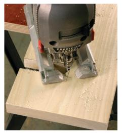
After making both of the long cuts, make a curved cut in the waste toward one of the corners. This will give you room to maneuver the saw to cut the end of the notch.
