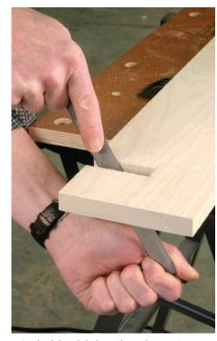
Using both hands helps to keep the rasp in a vertical position. Remove material evenly with long strokes of the rasp until you are down to the layout lines. Working to the lines will help you to keep the edges of the notches straight.
