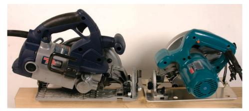
Not only can you see the difference between the worm drive saw (left) and the sidewinder (right), it is obvious that the sidewinder will be a lighter, more easily controlled saw.
