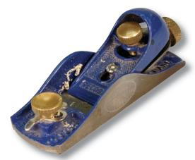
Block planes are commonly available. Paying a little more will add some nice features — a blade adjuster, a mouth that you can close up for high-tolerance work and the blade pitched at a lower angle. That said, even the cheap ones work well on softwoods when sharpened.
