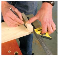
Measuring isn't always the best way to work accurately. Holding a block of scrap against the blade of the square guarantees that the line drawn will represent the thickness of the piece that will fit in the notch. It's much more important that the slot and the shelf be identical in size than it is to know the exact thickness of the shelf. Every time you measure and mark something you introduce the opportunity to make a mistake. I consider measuring to be a last resort, and avoid it when I can.
