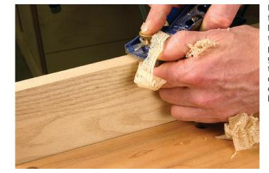
Note the grain on the face of the board. See how it is heading up toward the edge being planed? Think of those grain lines as fur. If the tool is pushing them down as it works, the chances are your cut will be sweet.
