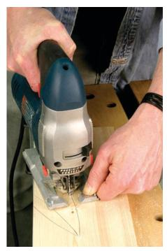
The jigsaw is a two-handed tool. A thumb on the baseplate will help steady the tool and will allow you great finesse as you round curves and track a line. We've removed the plastic guard on this saw (sorry, we shouldn't do that). With the guard in place, it's quite a feat to cut yourself.
