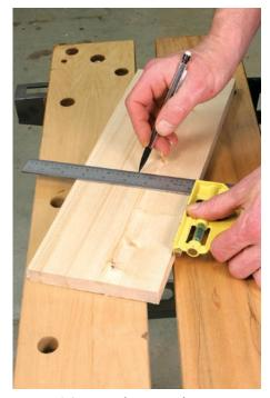
Accuracy is important here. Keep the square registered securely against the wood as you scribe the line. If anything feels like it shifted during scribing, make another line. Use a mechanical pencil to ensure your line is consistent in width.
