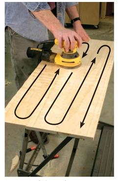
Move your sander in a regular pattern to ensure a consistent job. I'll start with overlapping strokes along the length of the board. Then I'll do overlapping strokes across the width. Then I repeat.
