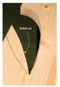
With a little practice you'll be able to cut very close to the line with your jigsaw. If you can leave just <sup>1/</sup>32" of waste, then it's simple work to rasp (or sand) down to your line. If you cross the line while cutting, you'll have no line to rasp to. Make a relief cut into the corner before cutting the curve.
