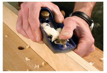
**3** • Use a block plane to remove the saw marks and create a square edge. Plane down to your cutting line (check both faces of your work).
