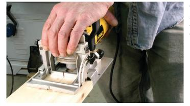
An alternate way to plunge: Squeeze the fence and tool handle together to make the cut.
