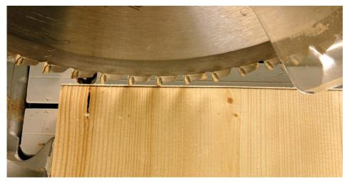
Here's a common operation with a miter saw – trying to remove just a bit to sneak up on a cutline. If you make this cut too fast (especially in hardwoods or thick stock), then the blade can deflect. Though it seems like you're making a light cut, slow down and take this operation a little slower than usual and check the cut across the thickness to ensure everything's OK.
