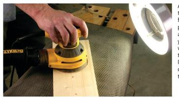
A raking light, such as the one shown here from a desk lamp, will point out the dings and scratches that your overhead lights will conceal. It helps to turn out your overhead lights as you sand critical areas (such as tabletops).
