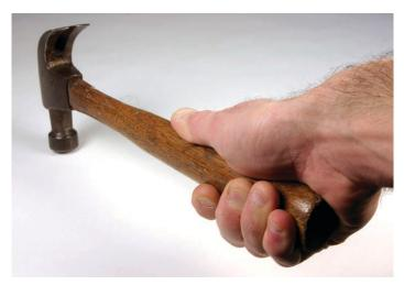
This is the power stroke with a hammer. When you build a deck, or really need to wallop something, grip the tool at the end of the handle. Sticking your thumb out will help steady the tool a bit.
