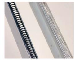
The teeth on the left are on the cheaper clamp. They're coarser and are only on a small portion of the bar. The teeth on the right are finer and there's more of them.
