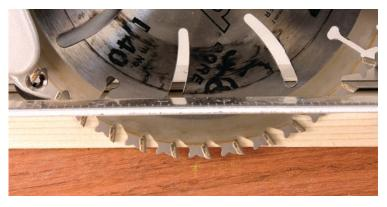
Properly setting the depth of cut will help extend the life of the blade and lessen the possibility of kickback.
