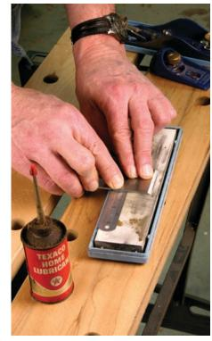
By propping up the back of the blade as you work the back, you'll greatly speed the polishing action of this critical surface. The ruler ensures that every time you do this it will be consistent.
