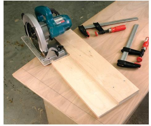
The jig has a wide fence to make clamping easy. Because this jig was created using the circular saw, whenever we clamp the jig exactly at the cut line, the result will be straight and on the layout line.
