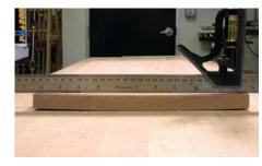
The use of the straightedge portion of the combination square will help to identify any cupping in the board. Return these boards to the stack and select another!
