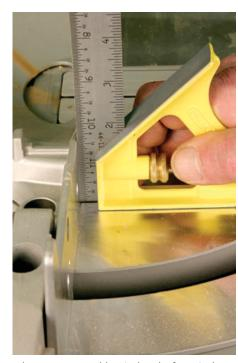
A less-common problem is that the fence isn't square to the table. Check this along several points on the fence. A twisted fence will wreak havoc with your accuracy.
