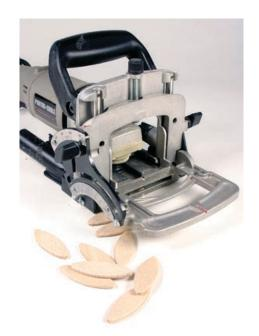
Biscuit joiners cut a football-shaped recess in two parts to be joined. The biscuits fit into that recess and (with a little glue) hold the joint together.
