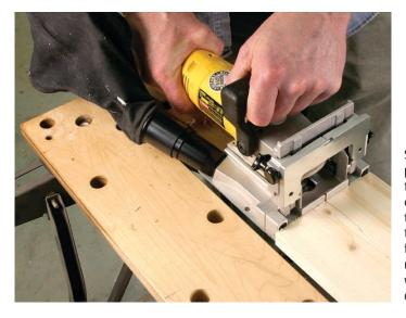
Some woodworkers prefer to work without the fence when they can. Here we're using the Workmate to control the tool instead of the fence. If you go this route, make sure your work surface is flat and debris-free.
