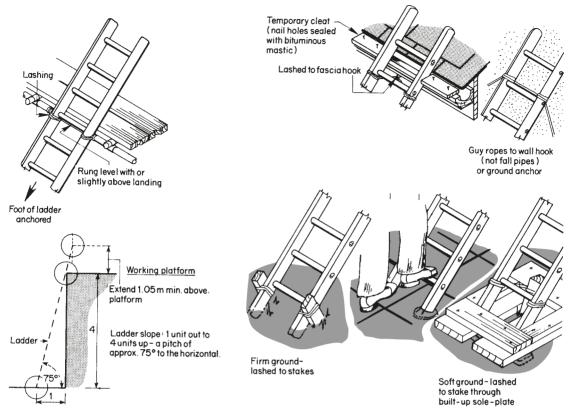
Fig. 10.4 Means of securing ladders
