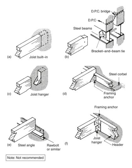
**Fig. 7.5** Joist bearings – abutting a wall (firring pieces not shown)
