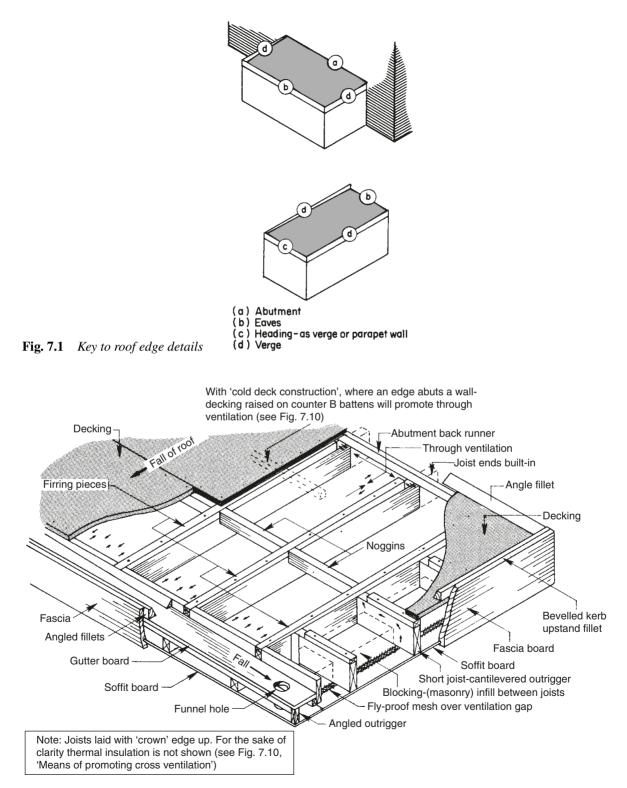
Fig. 7.2 Flat-roof construction (exposed isometric projection)
