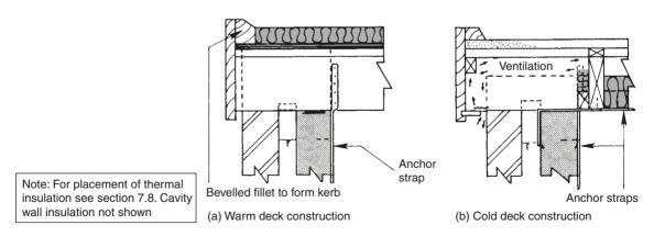
Fig. 7.7 Alternative verge details to a thermal-insulated roof (vertical section)
