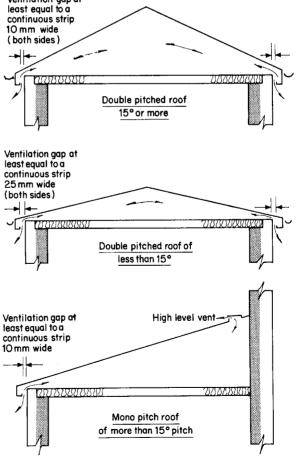
**Fig. 8.34** *Method of promoting cross-ventilation to a roof space*
