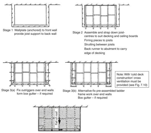
Roof plan Stage 4 Decking, insulation, soffits, fascia boards
