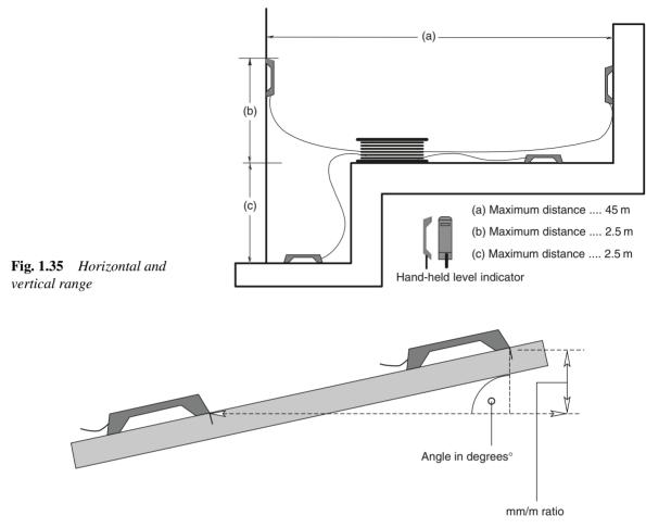
Fig. 1.36 Positioning the hand-held device to inclined surfaces
