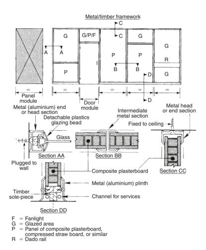
**Fig. 9.12** *Typical demountable partition system, using metal section, composite plasterboard panels, and glass*
