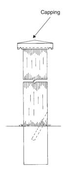
Fig. 2.22 Using capping
