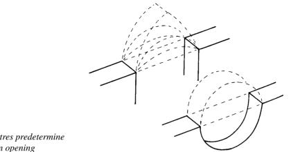
Fig. 4.2 *Centres predetermine* the shape of an opening
