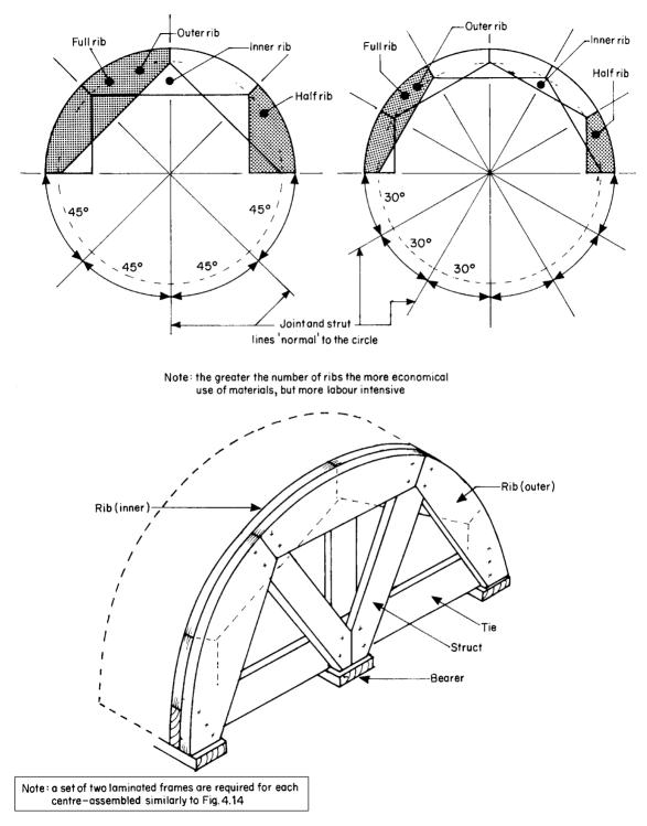
Fig. 4.15 Built-up rib construction
