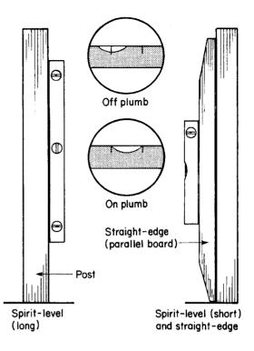
**Fig. 1.47** *Testing for plumb with a spirit level*
