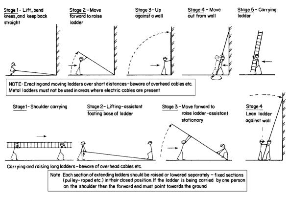
Fig. 10.3 Manipulating and manoeuvring ladders
