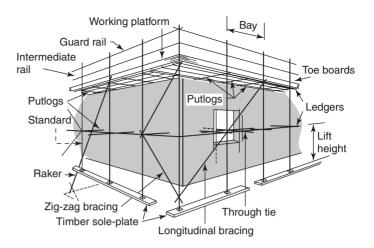
Fig. 10.10 Putlog-scaffold arrangement
