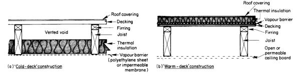
Fig. 7.11 Methods of providing thermal insulation
