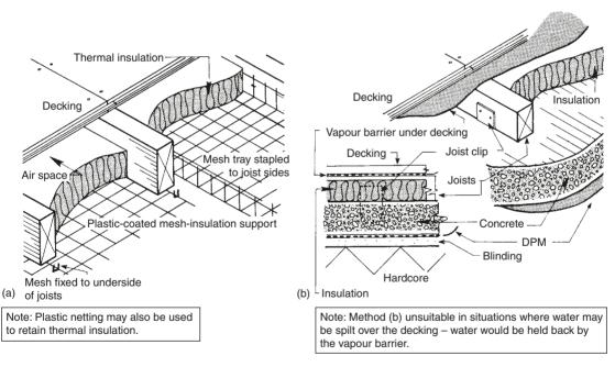
Fig. 5.20 Thermal insulation to ground floors
