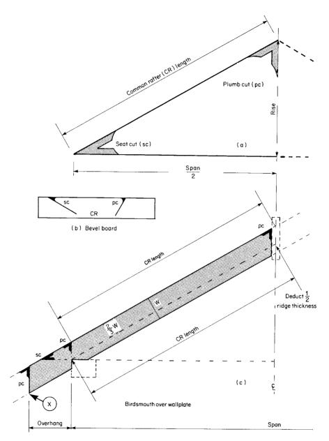
Fig. 8.5 Setting out for pattern rafter
