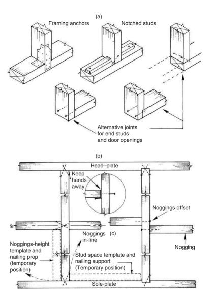
**Fig. 9.5** Joints and built-in framework
