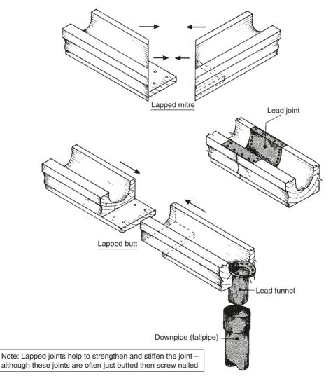
Fig. 8.36 Traditional wooden gutter joints and connections
