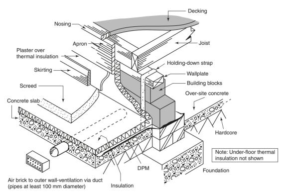
Fig. 5.15 Concrete-to-timber split-level floor
