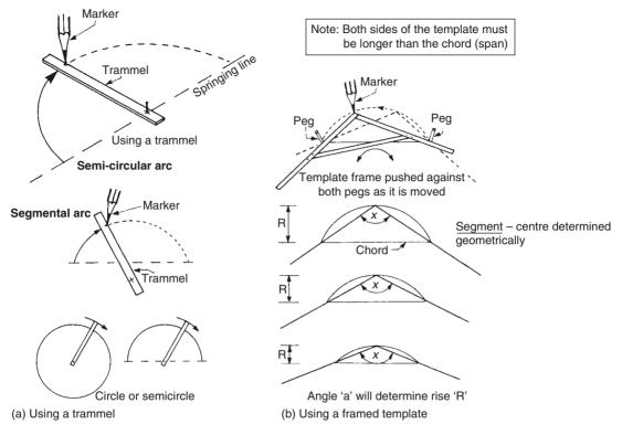
Fig. 1.26 Setting out large circles segments and arcs
