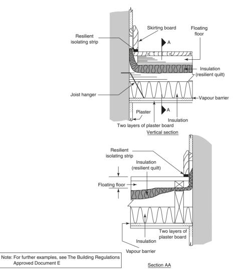
Fig. 6.15 Sound insulation to an upper floor
