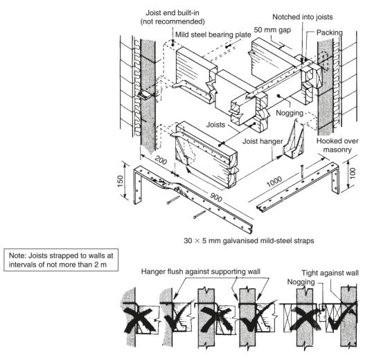
Fig. 6.2 Floor joist-bearing and lateral-wall support
