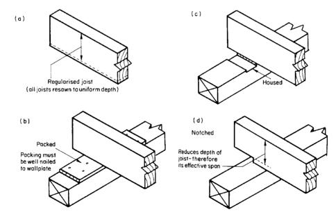
Fig. 5.7 Levelling and bearing adjustments
