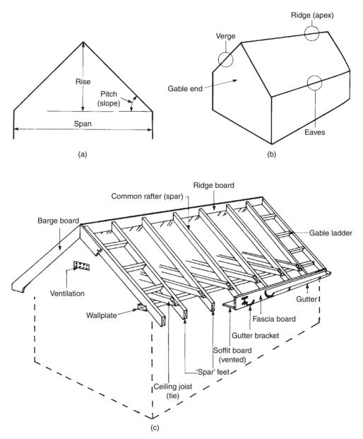
Fig. 8.1 Roof terminology (traditional roof)
