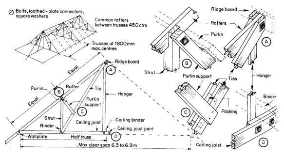
Fig. 8.20 TRADA domestic roof truss
