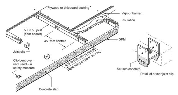
Fig. 5.16 Joists (floor bearers) to a concrete floor
