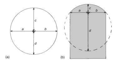
**Fig. 4.9** *Calculating the radii for an arc*
