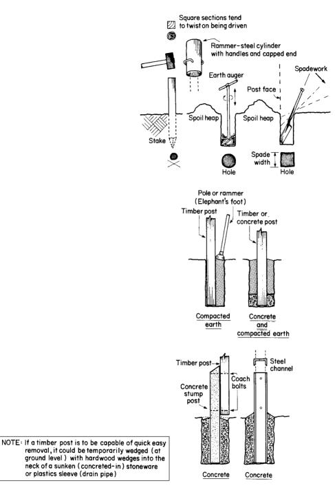
Fig. 2.19 Sinking and anchoring posts
