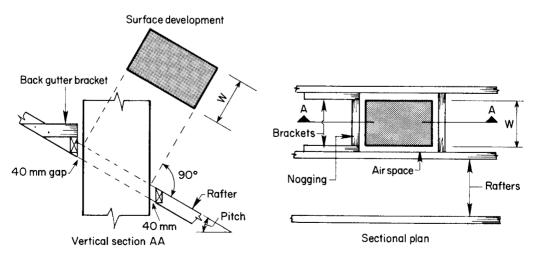
Fig. 8.30 Rectangular chimney stack or duct piercing a pitched roof
