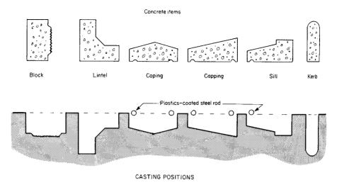
Fig. 3.1 Common pre-cast concrete products
