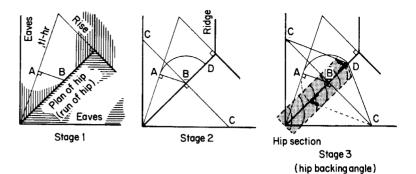
(ii) Draw line CC through B at right angles to the plan (run) of the hip. From B with compasses set to AB, scribe an arc to produce D.(iii) Join point D to C. The resulting angle will be the hip-backing
