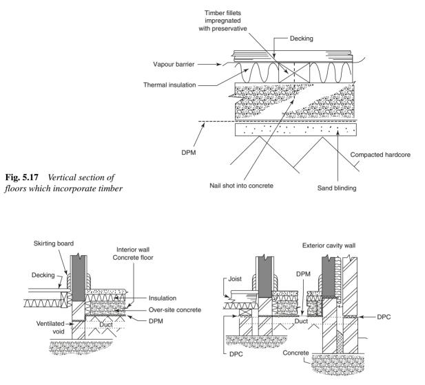
Fig. 5.18 Vertical section through timber and concrete floors adjacent to one another
