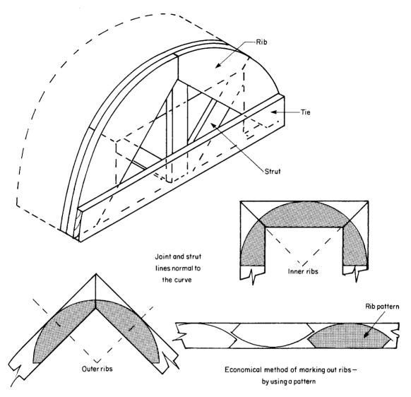
Fig. 4.16 Alternative built-up arrangement
