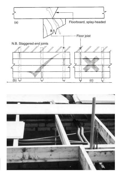
**Fig. 5.25** End jointing of floor boards
