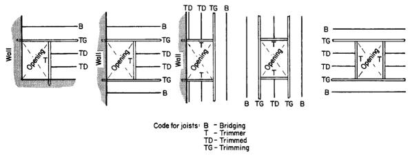
Fig. 6.4 Trimming floor openings – chimney breasts, wall protrusions, service traps, etc.
