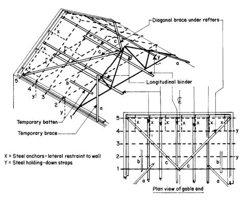
Fig. 8.26 Trussed-rafter-roof erection
