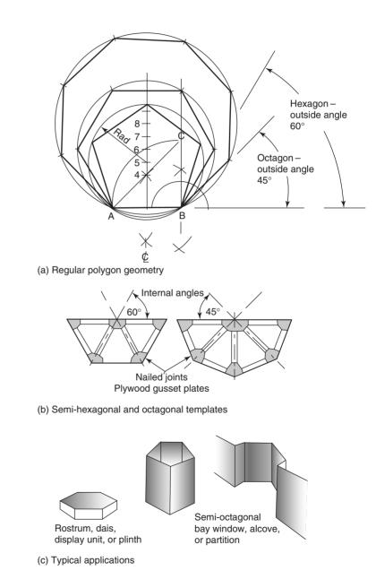
Fig. 1.23 Regular and semi-regular polygons and examples of use
