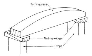
Fig. 4.10 Turning piece
