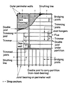
Fig. 6.1 Upper-floor joist layout
