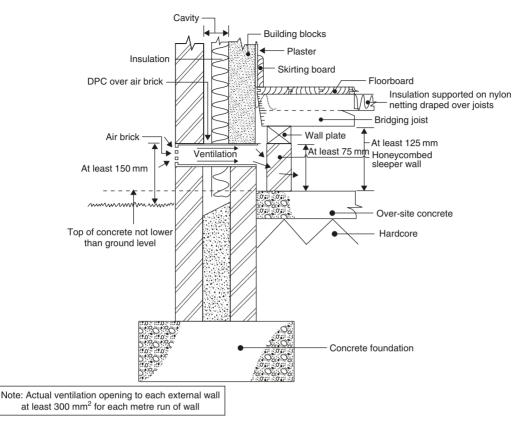
Fig. 5.2 Using sleeper walls to support floor joists
