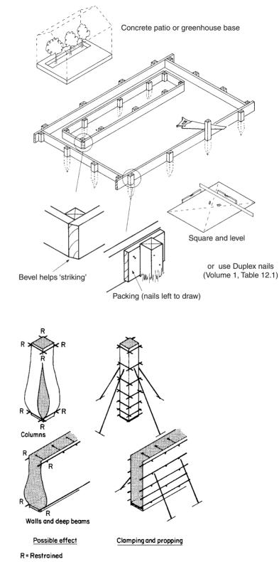
**Fig. 3.8** Formwork for an in situ concrete patio or base
