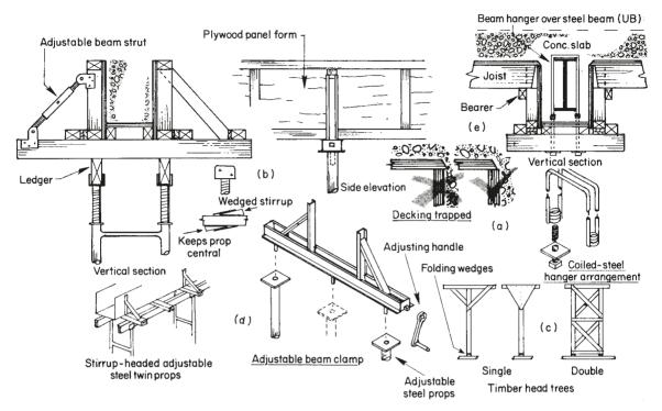
Fig. 3.19 Beam and lintel formwork
