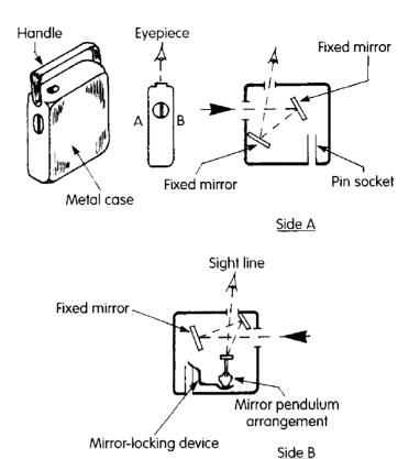
Fig. 1.37 Cowley level and mirror arrangement
