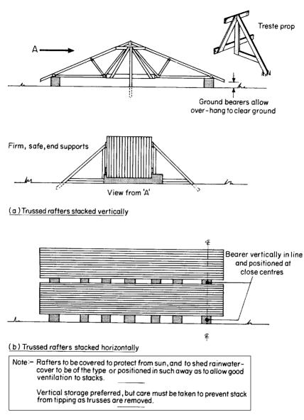
Fig. 8.24 Site storage of trussed rafters
