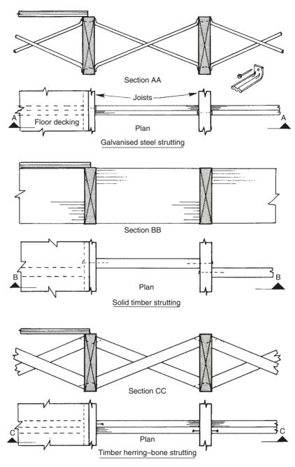
Fig. 6.9 Types of strutting
