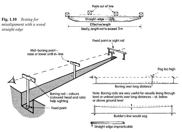
Fig. 1.11 Sighting or lining along a straight line over a long distance
