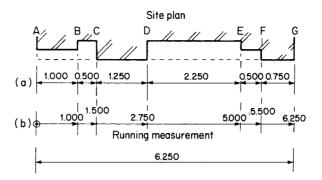
For example, an error between points B and C would result in points D, E, F, and G being wrongly positioned.
