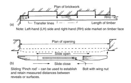
**Fig. 1.7** Useful devices for transferring measurements
