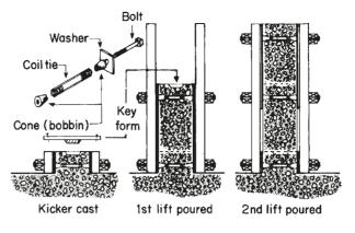
Fig. 3.15 *Climbing formwork*
