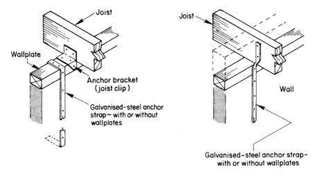
Fig. 7.8 Joist and wallplate anchorage
