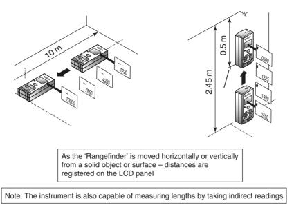
Fig. 1.5 Measuring distances using a Bosch Laser 'Rangefinder'
