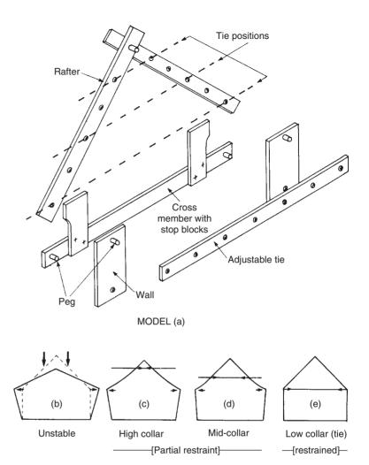
Fig. 8.4 Roof model, showing horizontal thrust
