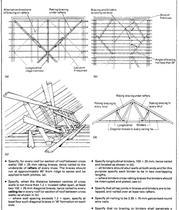
Specify (unless trusses are less than 5 m span), for every roof or section of roof between cross walls, 100 × 25 mm raking bracing twice nailed to every internal strut, (c).
