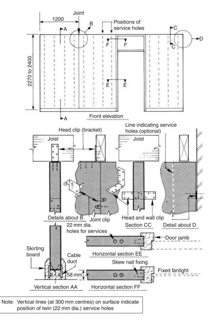
Fig. 9.13 Possible partition arrangement using the 'Karphos' non-demountable system
