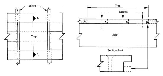
Fig. 5.27 Forming access and service traps
