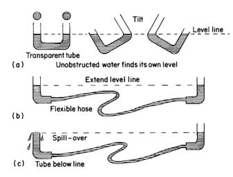
Fig. 1.31 Basic principles of a water level
