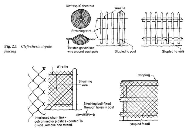
Fig. 2.2 Chain-link fencing (galvanised or plastics coated)
