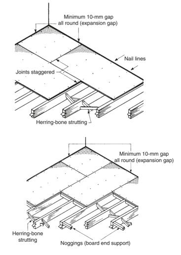
**Fig. 6.12** Laying tongued-andgrooved chipboard decking
