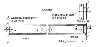
Figure 9.7(b) shows how a pre-assembled framework is wedged and packed-up off the floor before fixing. Where the head-plate falls between two ceilings joists, noggings are used as restraints and fixings.
