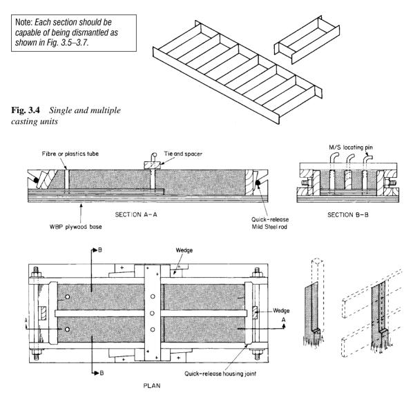
Fig. 3.5 Double mould box for pre-cast concrete posts
