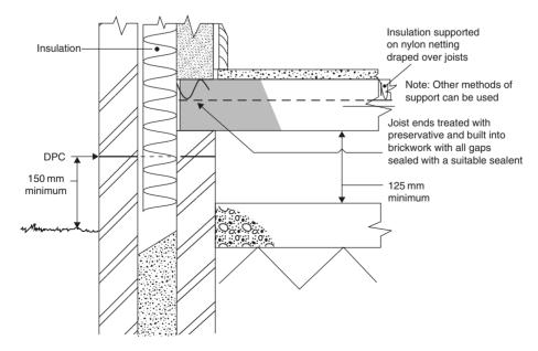
Fig. 5.3 Building-in floor joist (not recommended)
