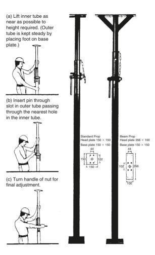
**Fig. 3.20** 'Acrow' adjustable steel props
