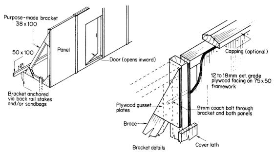
Fig. 2.10 Pre-fabricated panel and bracket
