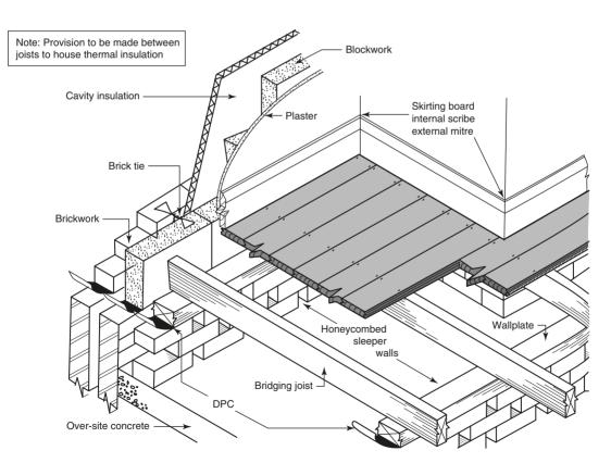
Fig. 5.1 Suspended timber floor
