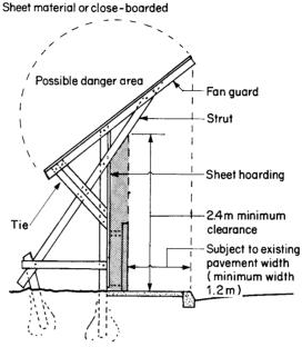
**Fig. 2.16** Fan hoarding: a diagrammatic representation
