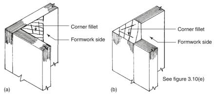
Fig. 3.11 Forming chamfers in column work
