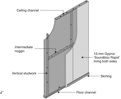
**Fig. 9.16** Exposed view of British Gypsum 'Gypwall Rapid' panel and fixing details
