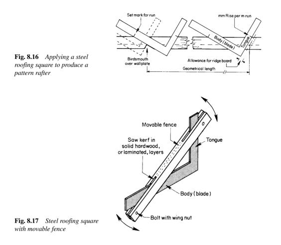
terms the square has been designed to cope with all the necessary roof bevels simply by using the roof's millimetre rise per metre run marking on the tongue and off-setting this against a 'set mark' (marked by an arrow) on the body to ascertain both the plumb and seat cuts as shown in Fig. 8.16. A purpose-made movable fence (Fig. 8.17) can make setting-up and angle transfers much easier. Proprietary 'buttons' are shown in Fig. 8.13.
