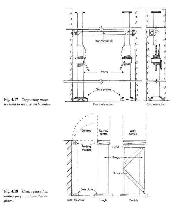
side of the opening. However, for thicker walls pairs of props on either side are recommended.
