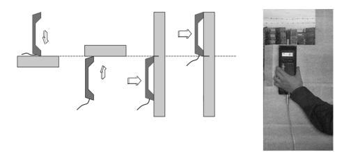
Fig. 1.34 Positioning the hand-held device
