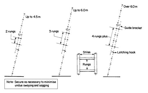
Fig. 10.2 Minimum rung-over-rung overlap for extending ladders (guide only)
