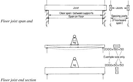
**Fig. 5.5** Floor joist end section in relation to its span
