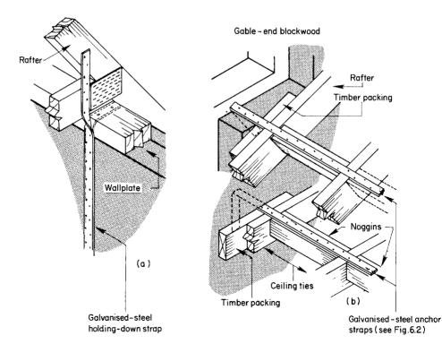
Fig. 8.29 Lateral support to a gable wall, and roof anchorage
