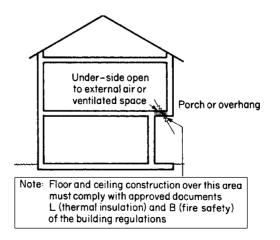
Fig. 6.14 Floors requiring thermal insulation
