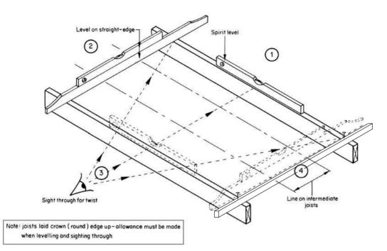
Fig. 5.6 Laying and levelling floor joists
