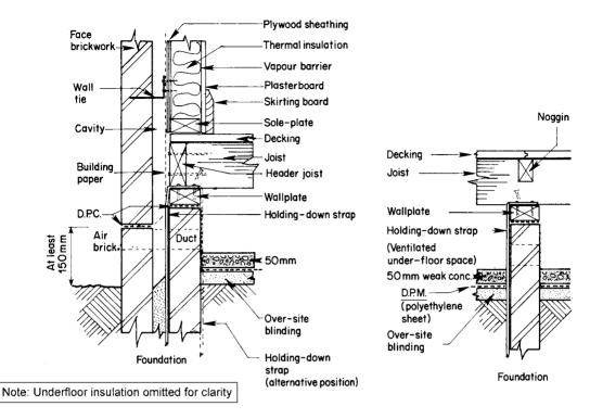
Fig. 5.8 Vertical sections through a floor to a timber-framed house
