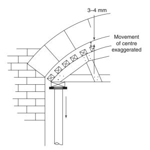
Fig. 4.19 Easing the arch centre
