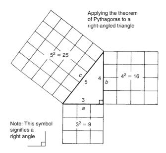
**Fig. 1.12** Using a ratio of 3:4:5 to form a right-angled triangle
