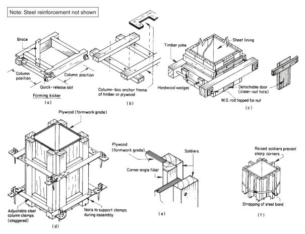
Fig. 3.10 Column-box construction and anchorage
