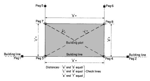
Fig. 1.20 Setting out a rectangular building plot
