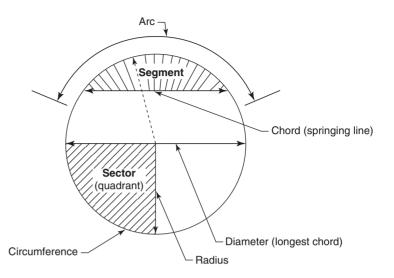
**Fig. 4.8** *Parts of a circle (also see Volume 1, Fig. 1.20)*
