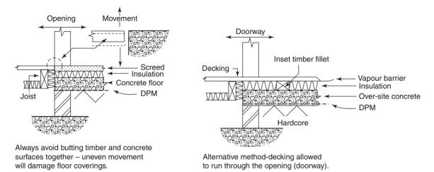
Fig. 5.19 Vertical sections to show abutting timber to concrete floors
