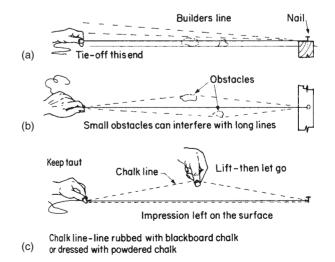
**Fig. 1.9** Using a builder's line to leave a straight chalk line impression on a flat surface
