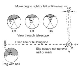
**Fig. 1.16** *Setting out a right angle with an optical square*
