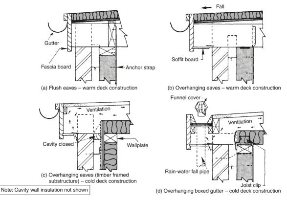
**Fig. 7.6** Alternative eaves details to a thermal-insulated roof (vertical section). Cavity wall insulation not shown
