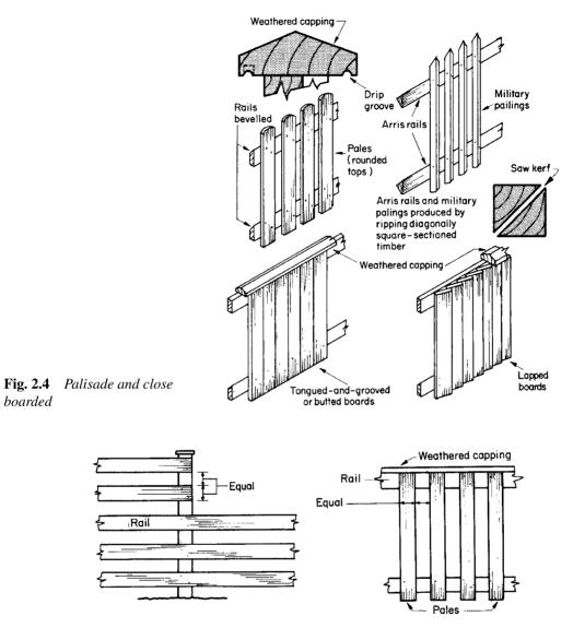
Fig. 2.5 Ranch fencing (boards and gaps of equal width)
