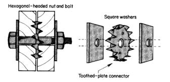
Fig. 8.21 Toothed-plate connection (double-sided connector)
