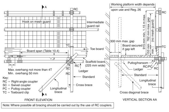
Fig. 10.16 Working platform for a tubular scaffold
