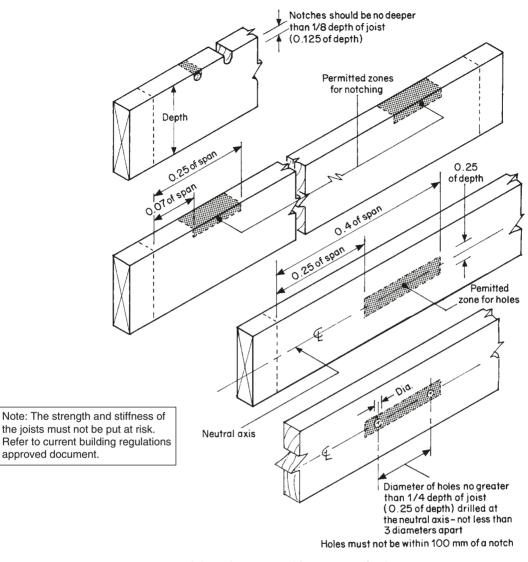
This information is a general ( rule of thumb ) guide only – for single family houses of not more than 3 storeys, and where joists donot exceed 250mm depth
