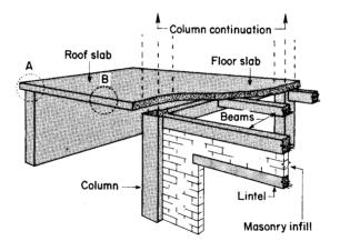
Fig. 3.2 *Key to* in situ *structural elements*
