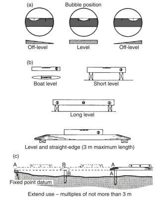
Fig. 1.29 Levelling with a spirit level
