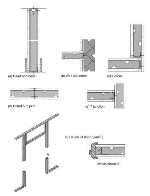
Fig. 9.15 'Gypwall Rapid' Non-demountable system
